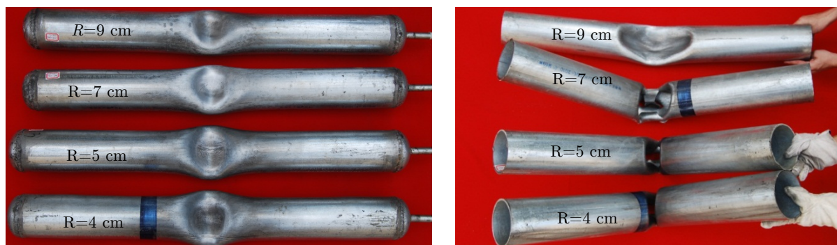
(d) 200g TNT charge and 2.75mm thickness.
