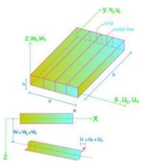
Figure 1: Illustrations of displacements and plate meshing arrangement.
