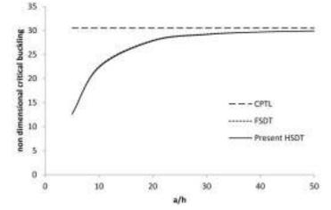
Figure 13: The effect of side-to-thickness ratio on nondimensionlized uniaxial buckling load of simply-supported four-layer (0 / 90 / 0 / 90) square laminates subjected to uniaxial buckling;  $E_1/E_2 = 40$ .
