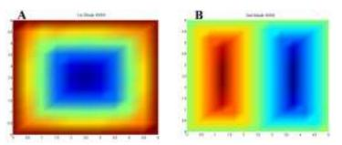
Figure 10: The first two buckling mode shapes of a square orthotropic plate with simply supported boundary conditions.
