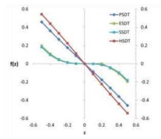
**Figure 2:** Variation of functions  $f_i(z)$  along the plate thickness.
