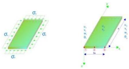
Figure 4: Pre-buckling stresses in a strip.
