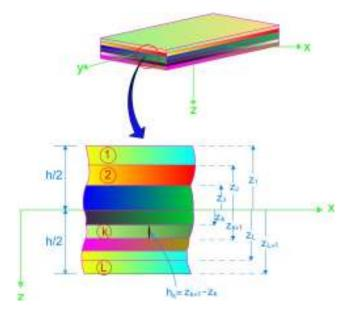
Figure 3: Coordinate system and layer numbering used for a typical laminated plate.
