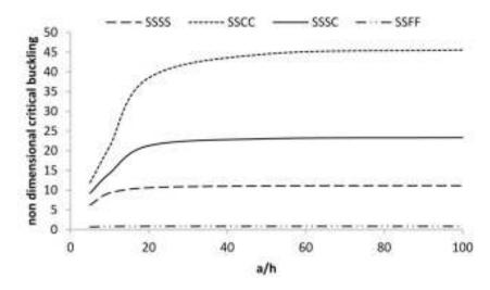
Figure 11: The effect of side-to-thickness ratio on the critical buckling load of square plates with different boundary conditions subjected to uniaxial compression along the y-axis;  $E_1/E_2 = 10$  and PSDT model.
