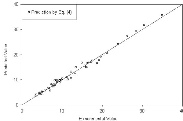
Figure 3: Prediction of dimensionless maximum permanent deflection by regression model (60 data points)
