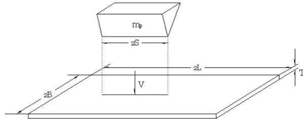
Figure 1: A fully clamped rectangular plate struck by wedge at the centre of the plate
