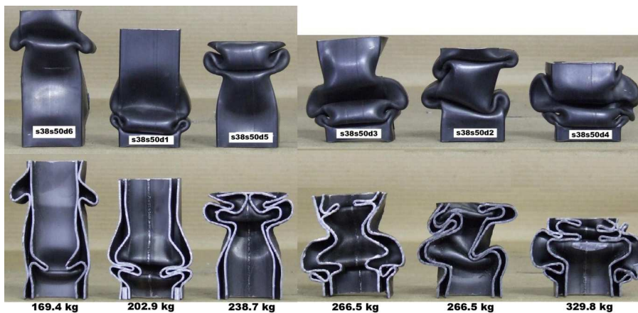
Figure 25: Side and section view of dynamically crushed s38s50
