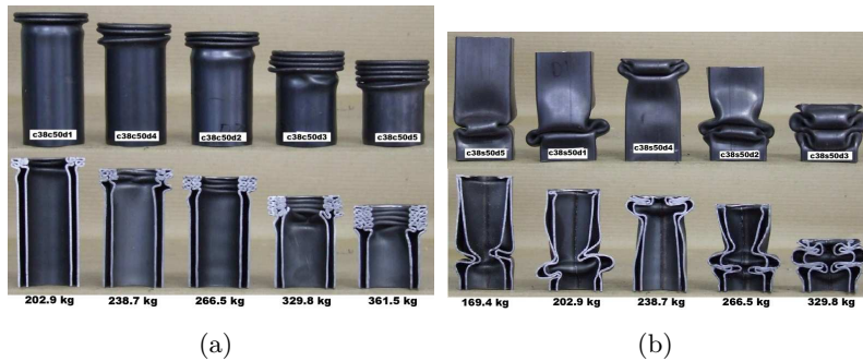
Figure 24: Side and section view of dynamically crushed (a)c38c50 (b)c38s50
