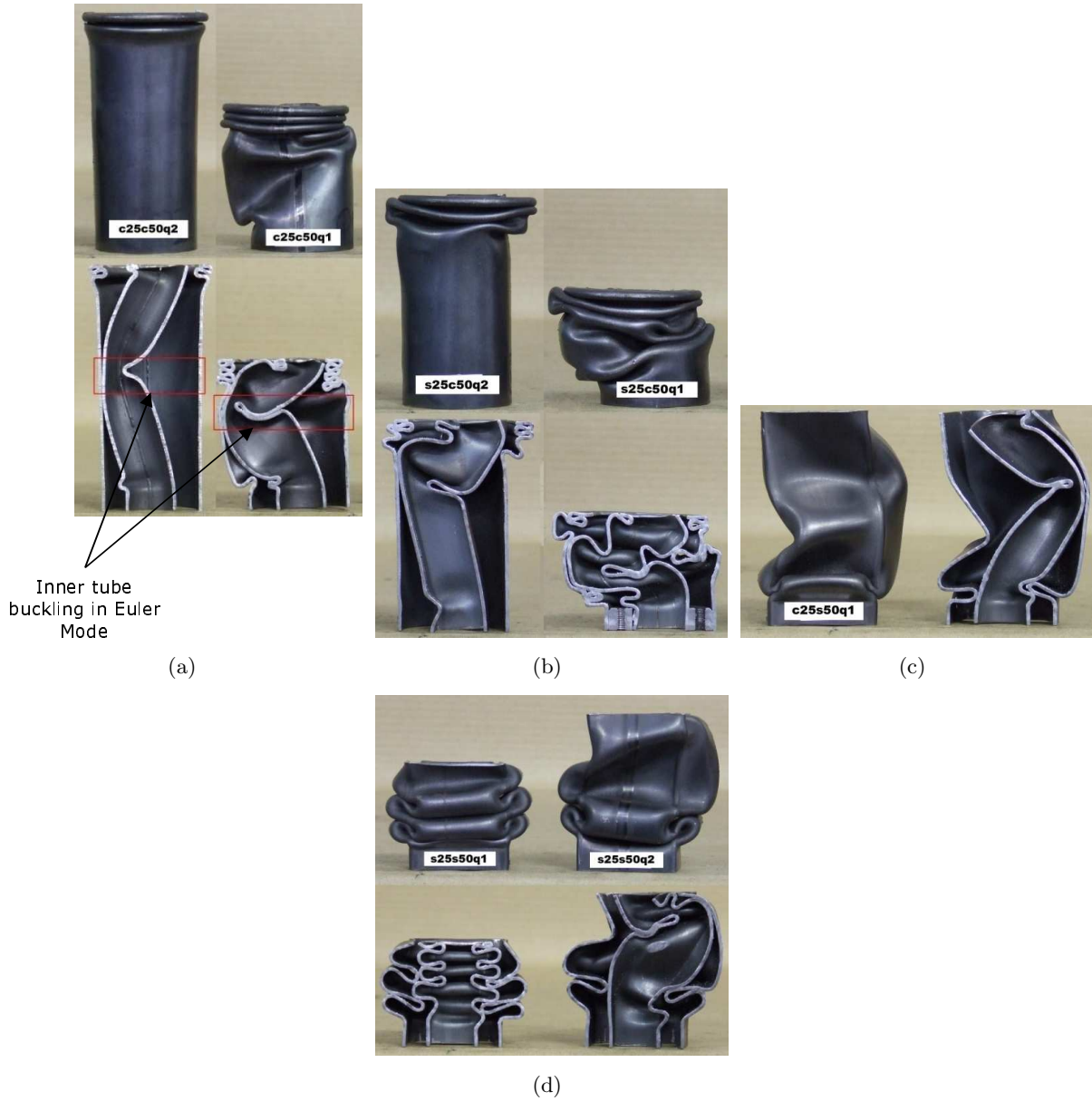
Figure 6: Side and section view of quasi-statically crushed (a) c25c50 (b) s25c50 (c) c25s50 (d) s25s50.
