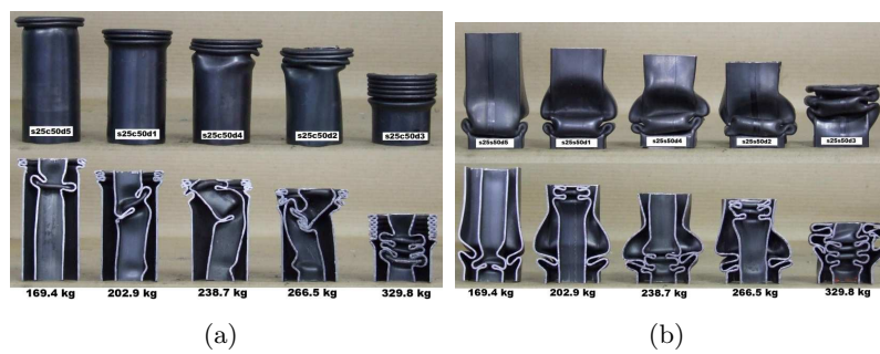
Figure 23: Side and section view of dynamically crushed (a)c25s50 (b)s25s50
