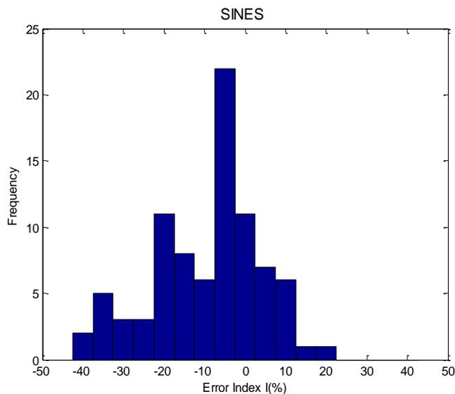
Figure 2: Histogram of fatigue index error for Sines criterion.
