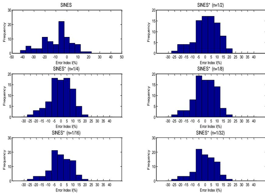
Figure 4: Histograms of fatigue index error for Sines and modified Sines criteria.
