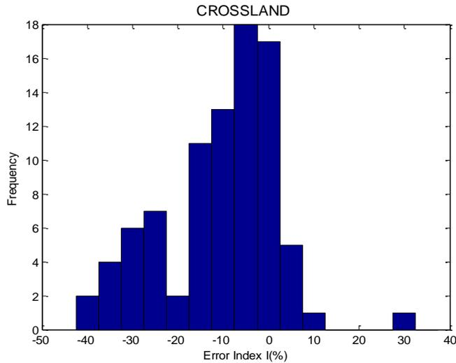
Figure 1: Histogram of fatigue index error for Crossland criterion.
