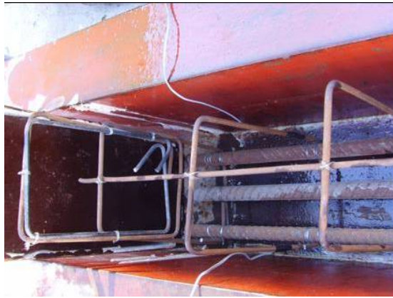
Figure 8 A view of Group-2 specimens' reinforcement from inside the mould.
