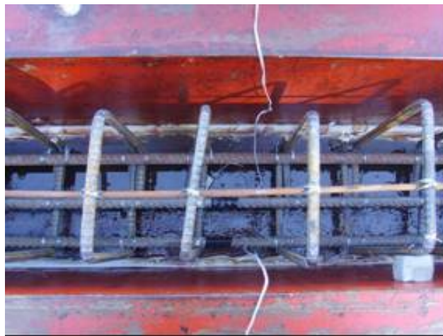
Figure 7 A view of Group-1 specimens' reinforcement from inside the mould.
