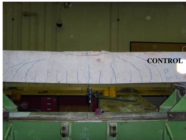
Figure 16 Flexural failure of Group-1 control beam specimen.
