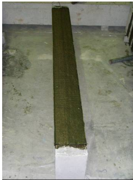
Figure 10 Beam strengthened with CFRP sheet only (Group-1, scheme -1).
