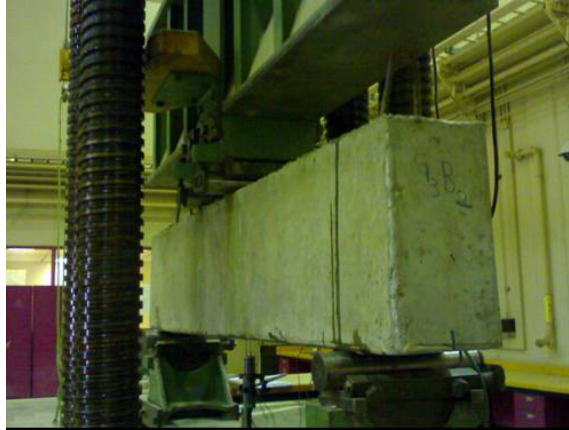
Figure 13 Test set up used for testing of beam specimens.
