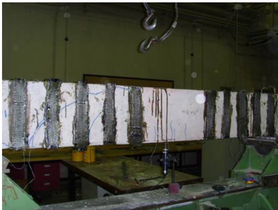
Figure 23 Failure of vertical strip strengthened RC beam specimen (Group-2, Scheme-1).
