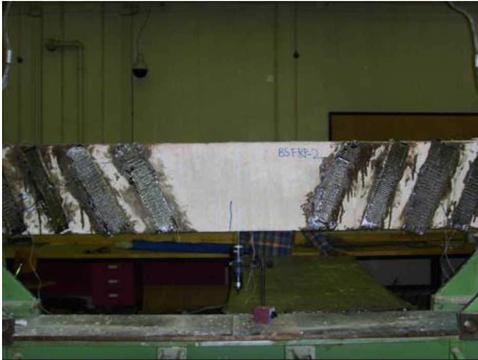
Figure 24 Failure of inclined strip strengthened RC beam specimen (Group-2, Scheme-2).
