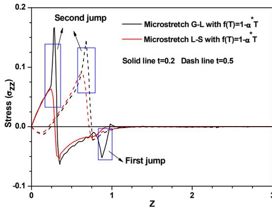
Figure 5: Stress ( $\sigma_{zz}$ ) distribution at  $x=0$  versus  $z$  under different generalized thermoelastic theories.
