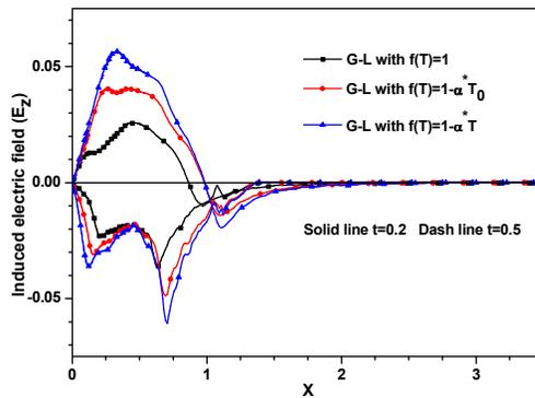
Figure 14: Induced electric field ( $E_z$ ) distribution at  $z=0$  versus  $x$  under different forms of temperature dependent material properties.
