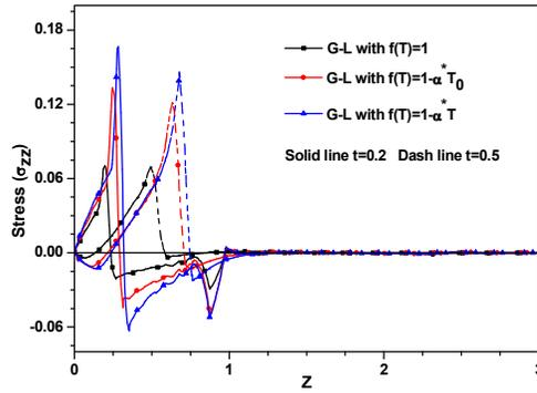
Figure 12: Stress ( $\sigma_{zz}$ ) distribution at  $x=0$  versus  $z$  under different forms of temperature dependent material properties.
