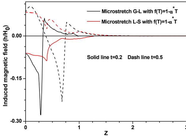
**Figure 7:** Induced magnetic field ( $h/H_0$ ) distribution at  $x=0$  versus  $z$  under different generalized thermoelastic theories.
