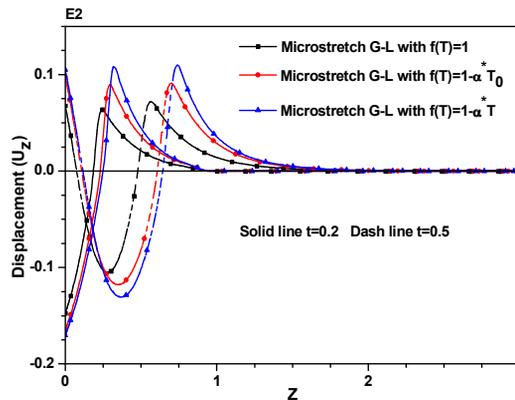
Figure 11: Displacement ( $U_z$ ) distribution at  $x=0$  versus  $z$  under different forms of temperature dependent material properties.
