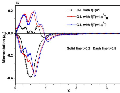
Figure 13: Microrotation ( $\phi_y$ ) distribution at  $z=0$  versus  $x$  under different forms of temperature dependent material properties.
