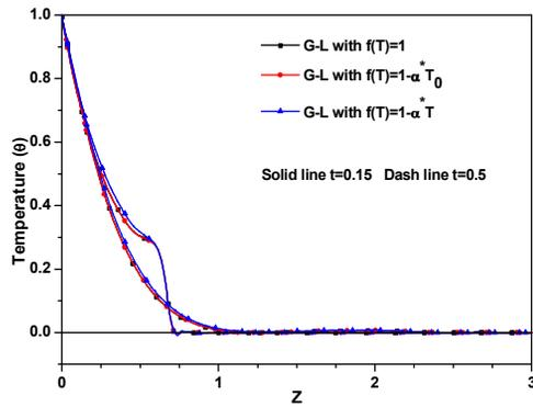
Figure 9: Temperature ( $\theta$ ) distribution at  $x=0$  versus  $z$  under different forms of temperature dependent material properties.
