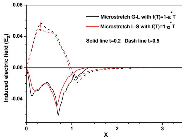
**Figure 8:** Induced electric field ( $E_z$ ) distribution at  $z=0$  versus  $x$  under different generalized thermoelastic theories.
