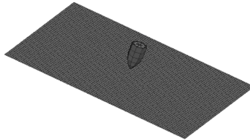
Figure 1 Plate modelled with shell elements and projectile with solid elements.
