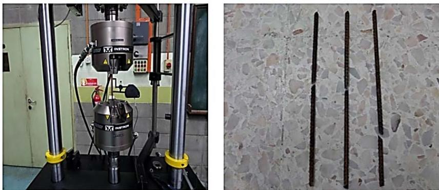
Figure 3: Test set-up and tested mesh specimen.
