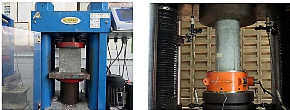
Figure 4: Cube and Cylinder test of concrete.
