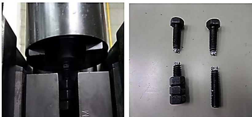
**Figure 2:** Test set-up and tested bolt specimen.
