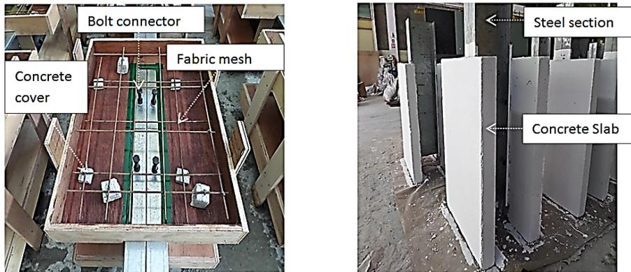
Figure 7: Push-out test specimens before and after casting.
