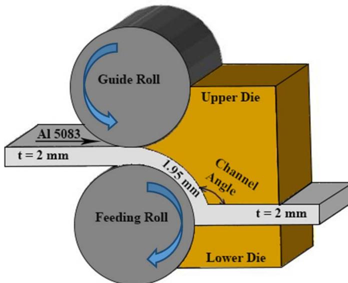
Figure 1: schematic of ECAR process.
