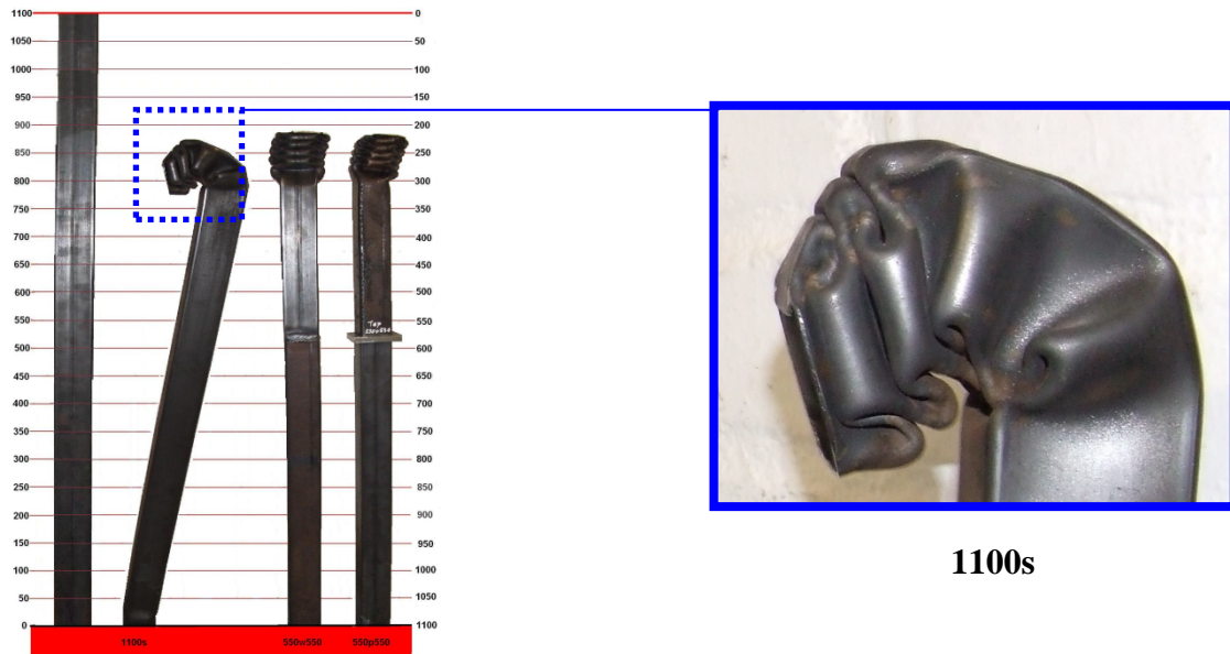
Figure 16 Buckling profiles of 1100mm specimens with close-up of 1100s showing initial progressive buckling and subsequent global buckling characterising transition buckling.
