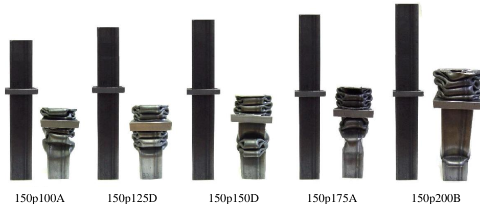
Figure 11 Plate-divided specimens with L_{bottom} = 150\text{mm} and L_{top} ranging from 100mm to 200mm in 25mm increments. h = 3.26\text{m} .
