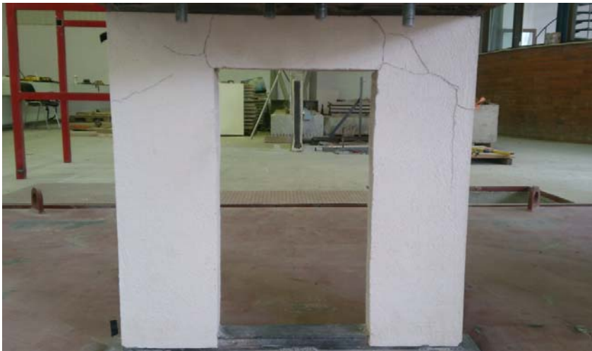
Figure 14: Final deformation and crack states at the end of experiment in Example 2.
