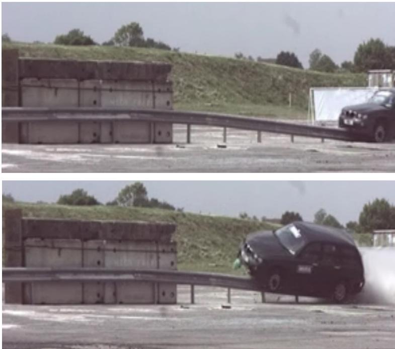
**Figure 2:** Accident pictures of a vehicle hitting a bridge pier after impacting a 12 m long TDGET (Powell, 2012).
