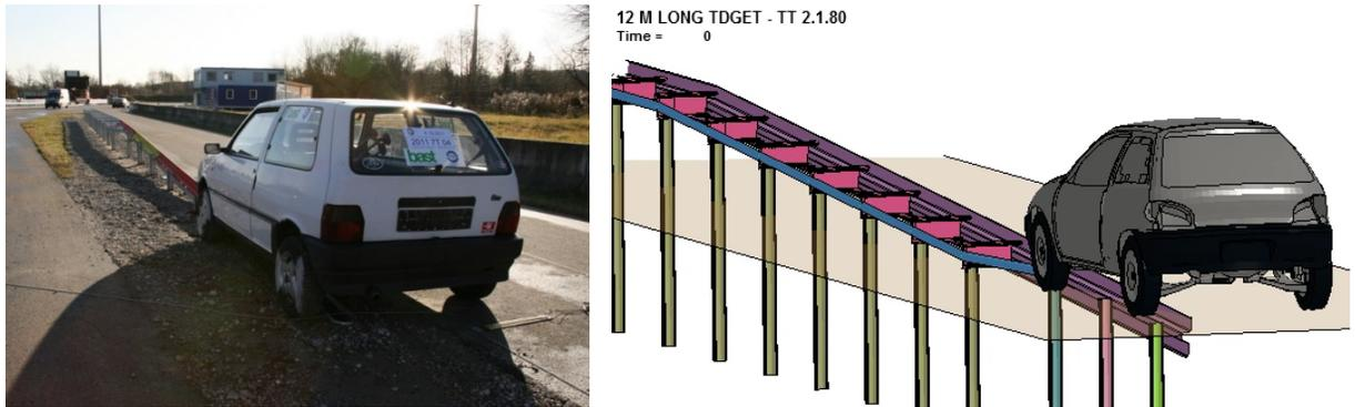
**Figure 7:** Position of the 900 kg car before test TT 2.1.80
