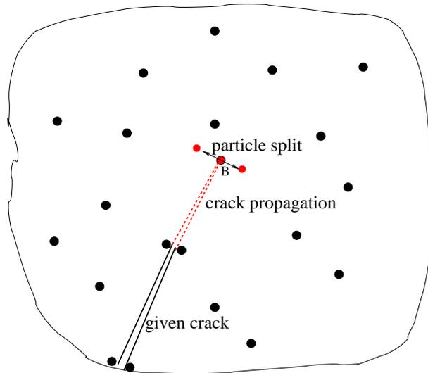
Figure 5: Scheme of crack propagation and particle split
