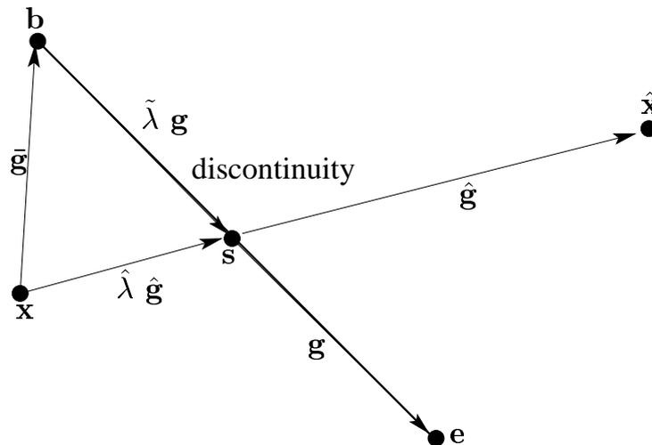
Figure 4: A crack modelled with the visibility criterion
