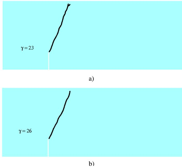
Figure 20: Crack pattern of the John and Shah beam under impact loading for a location of the notch:  $x=5.08\text{cm}$ , a) for the  $dcm_2$  model (with circular refinement), b) for the  $dcm_1$  model (without circular refinement)
