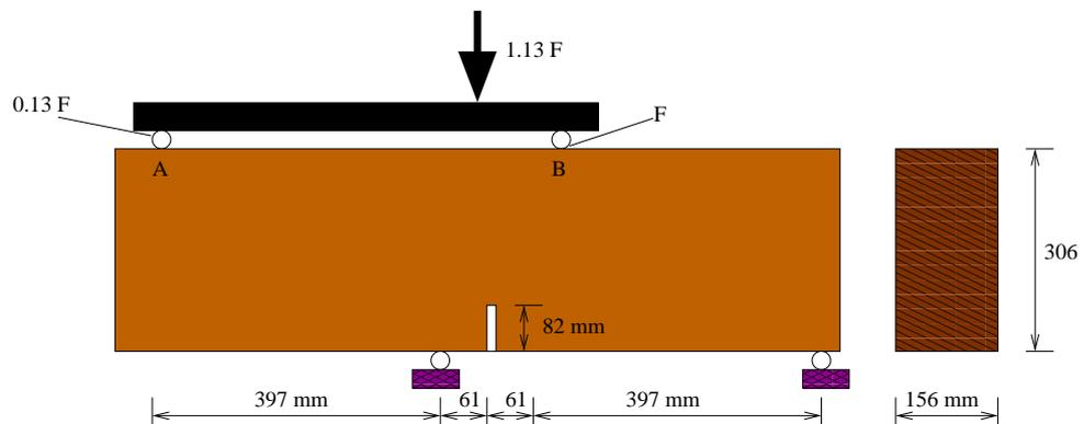
Figure 14: The tensile/shear beam from Arrea and Ingraffea
