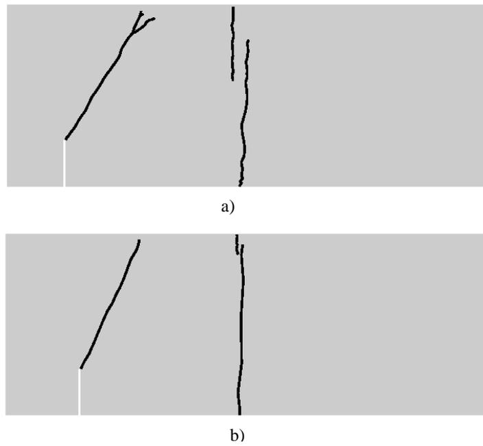
Figure 22: Computed crack pattern of the John and Shah beam near the transition in the failure mode, a) under quasistatic loading, b) under dynamic loading
