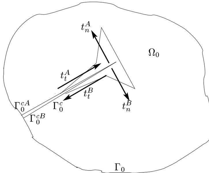
Figure 1: Domain with crack boundary
