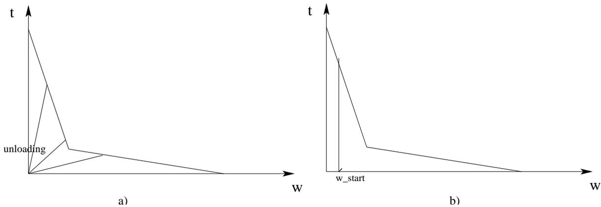
Figure 12: Discrete crack model
