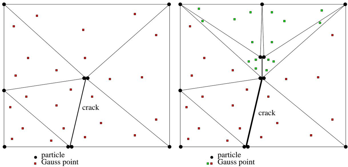
Figure 8: Crack propagation scheme and triangulation using an integration scheme based on a background mesh
