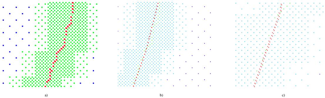
Figure 17: Crack pattern for a cutout of the beam for a) without circular refinement, b) with circular refinement for a refinement radius of  $r = 0.95 \delta x$ , c) with circular refinement with  $r = 0.5 \delta x$
