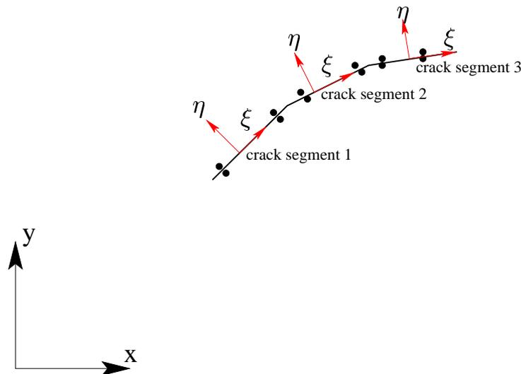
Figure 11: Relation between local crack coordinate system and global coordinate system
