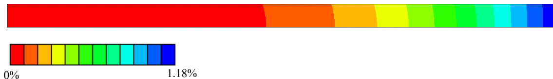
Figure 8: Numerical prediction of the moisture profile of XNR 6852-1 after 24 hours of ageing.
