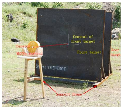
Figure 11: Experimental setup of MEFP warhead against 45# steel target.
