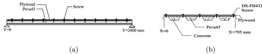
Figure 3 Structural model of the PSSDBC system (a) Longitudinal section (b) Transverse section.
