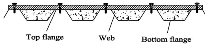
Figure 9 Illustration of supports under top & bottom flanges and web of the PSS.
