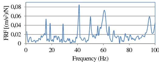
Figure 7 Experimental estimation of FRF between excitation at point A and response at point B (Note: The points A and B were selected in  $y=1200$  and  $y=2200$  mm (figure 3.a) respectively, along the length and middle point of width for PSSDBC panel).
