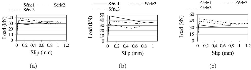
Figure 5 Load-Slip curves between Peva45 and (a) C25 (b) C30 (c) C35.
