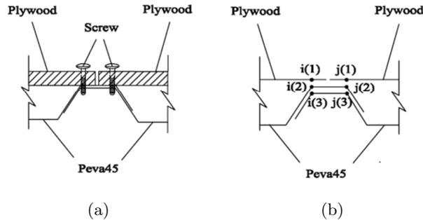
Figure 14 Detail A: (a) Constructional model (b) Analytical model.
