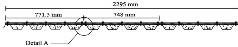
Figure 12 The PSSDBC panel with three repeating sections.
