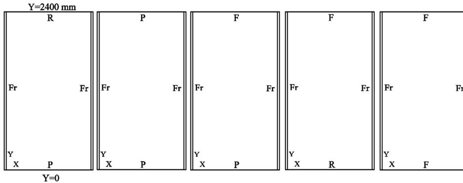
Figure 8 Various end support conditions perpendicular to the strong direction of the PSS (*Fr = Free*).
