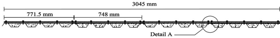
Figure 13 The PSSDBC panel with four repeating sections.
