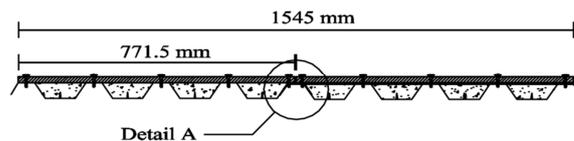
Figure 11 The PSSDBC panel with two repeating sections.
