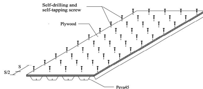
Figure 1 Profiled steel sheet dry board system.
