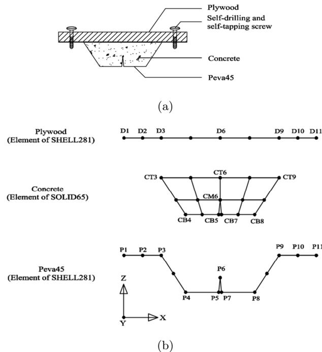
Figure 6 (a) One bay PSSDBC structural system (b) Situation of nodes in elements of one bay PSSDBC system.
