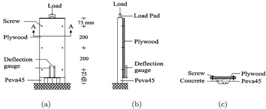
Figure 4 Detailed arrangements of the push-out test: (a) Front view (b) Side view (c) Section A-A.
