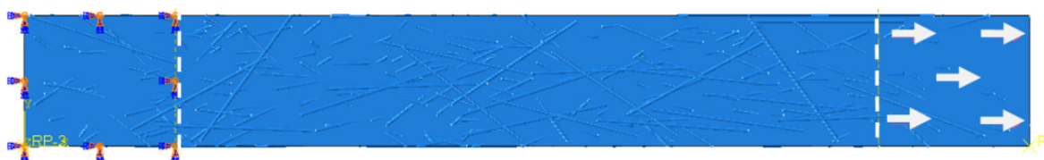
Figure 4: FEA Tensile Test Loading and boundary conditions.
