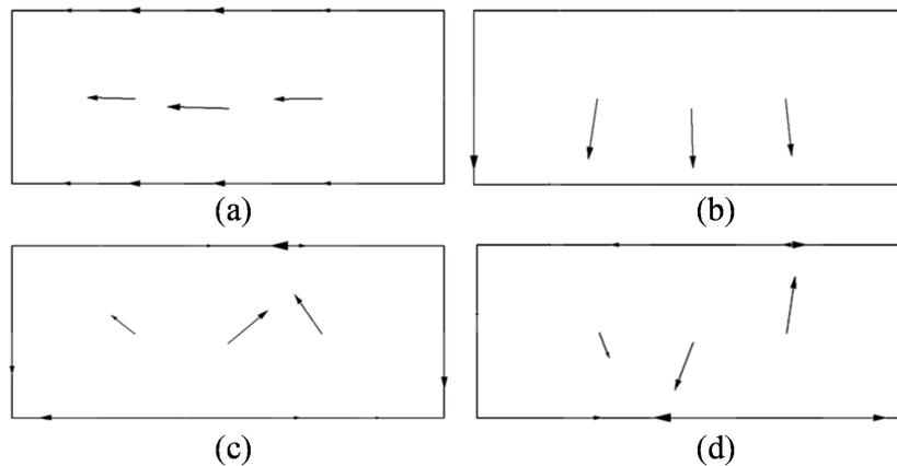
Figure 4 Spurious modes appearance in a rectangular cavity. (a) First longitudinal mode. (b) First vertical mode ( $3^{rd}$  mode). (c-d)  $5^{th}$  and  $6^{th}$  modes with a high rotational tendency.
