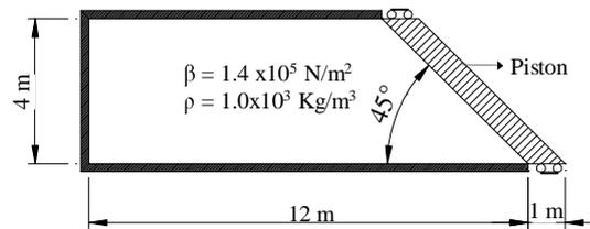
Figure 5 Skewed cavity coupled with movable piston.
