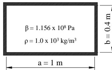
Figure 2 Rectangular cavity. Dimensions and fluid properties.
