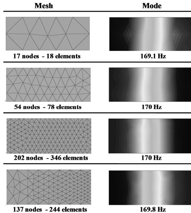
Figure 3 Rectangular cavity results. Meshes at left. Pressure distribution for the 1<sup>th</sup> mode at right.
