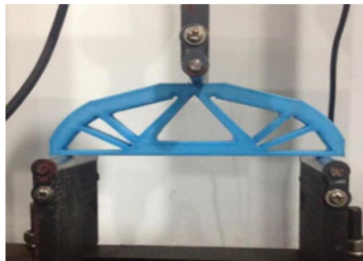
Figure 21: The loading and supporting condition on the tensile machine for MBB beam.
