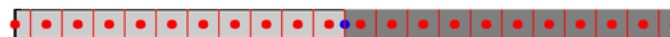
Figure 5: 1D bi-material bar. Domain discretization and corresponding finite volumes. Blue and red dots are denoted the enrichment node and field nodes, respectively. 1D local background finite volumes are illustrated by red lines.
