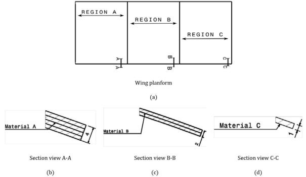
Figure 6: Wing Planform showing various sections highlighting the thickness and material lay-ups
