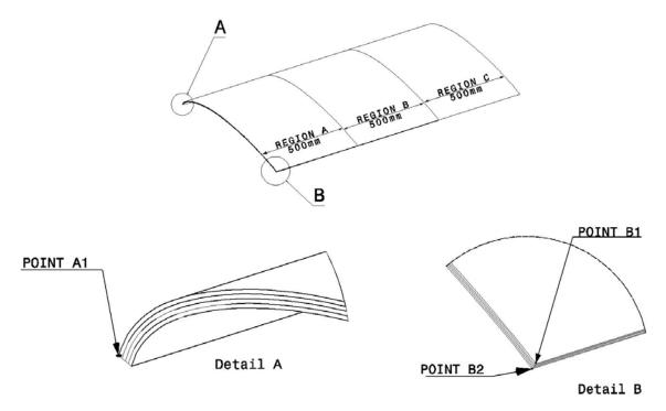
Figure 5: Wing Planform showing Boundary conditions Points
