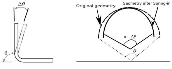
Spring-in of corner sectionsSpring-in of curved panelsFigure 1: Spring-in of corner sections and curved panels
