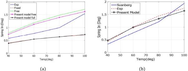
Figure 4: Comparison of Svanberg's plane strain results with the 3D results
