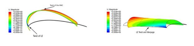
(a) (b) *Figure 8:* Displacement plots of Wing A showing twists and Warpage.
