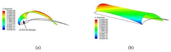
Figure 9: Displacement plots of Wing B showing twists and Warpage.
