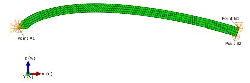
*Figure 7: Finite Element Mesh and Boundary condition points of the wing root section.*
