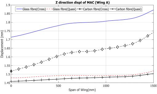
Figure 11: MAC Z direction displacement plots of Wing A
