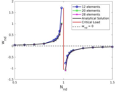
**Figure 6:** Critical load of a simply supported square plate  $N_v = N_{cr}$  and  $N_x$  variable.
