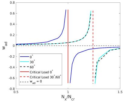
Figure 17: Critical buckling load of a simply supported square plate with ply-orientation angles of 0°, 30° and 60°.
