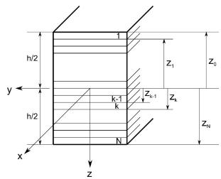
Figure 2: A symmetric laminated composite with N plies.
