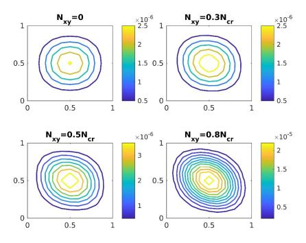
Figure 12: Displacement isocurves of a clamped square plate.
