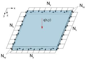
Figure 1: Compressed plate.
