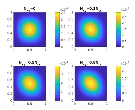
Figure 13: Displacement fields of a clamped square plate.
