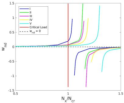
Figure 18: Critical buckling load for beveled orthotropic plates
