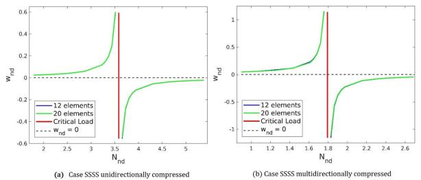
Figure 15: Critical buckling loads for orthotropic plates
