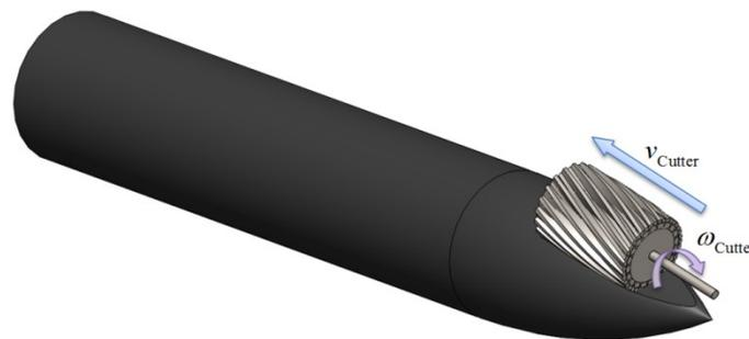
Figure 1: Manufacturing process of U-shape-nose grooved projectile
