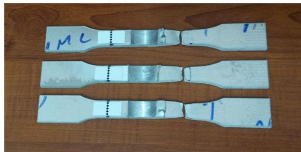
Figure 11: Fracture positions of the as-welded test specimens
