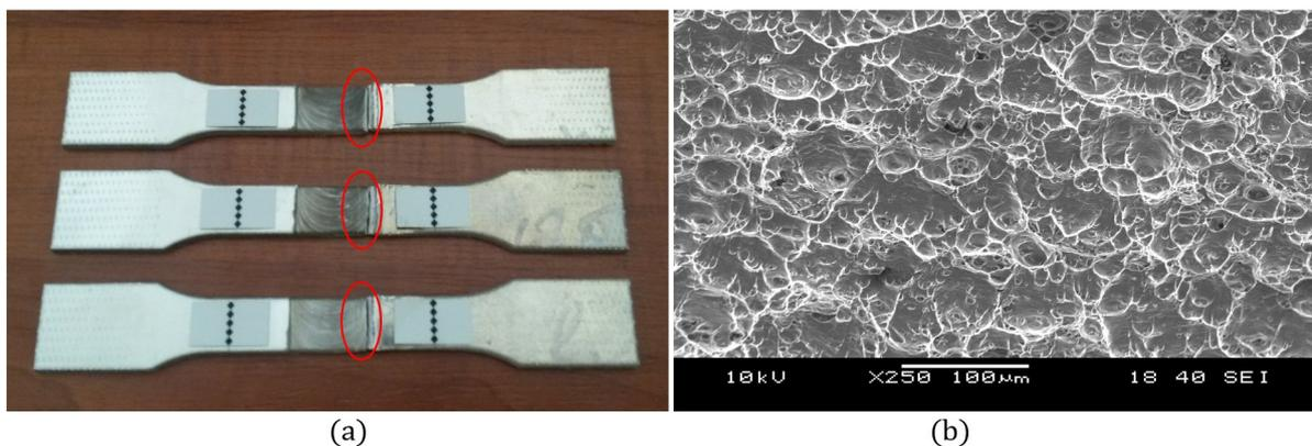
Figure 13: PWHT specimens: (a) failure positions (b) SEM fractography
