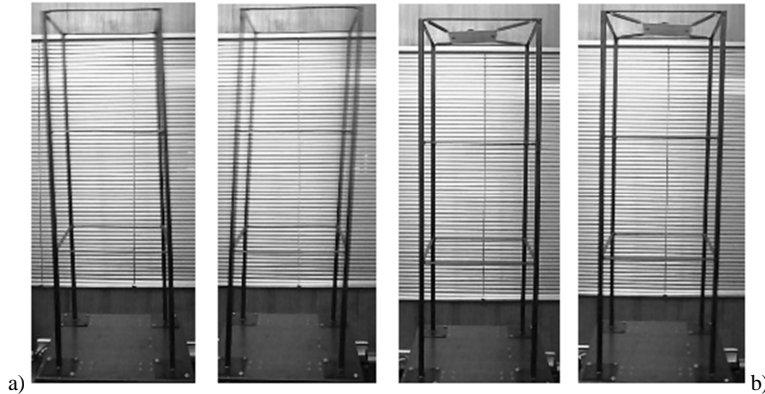
Figure 13 Frames showing structure responses during forced vibration at frequency 8 Hz and imposed amplitude of 1 cm: a) without and b) with absorber.
