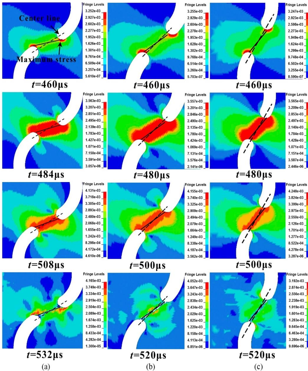
**Figure 9:** Von-Mises stress distribution (the stress values are in 100GPa) of specimens during fracture process. (a) 30°. (b) 45°. (c) 60°.
