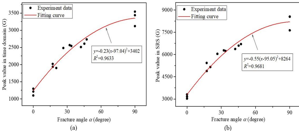
**Figure 13:** Peak acceleration versus fracture angle. (a) Peak values in time domain. (b) Peak values in maximum SRS.
