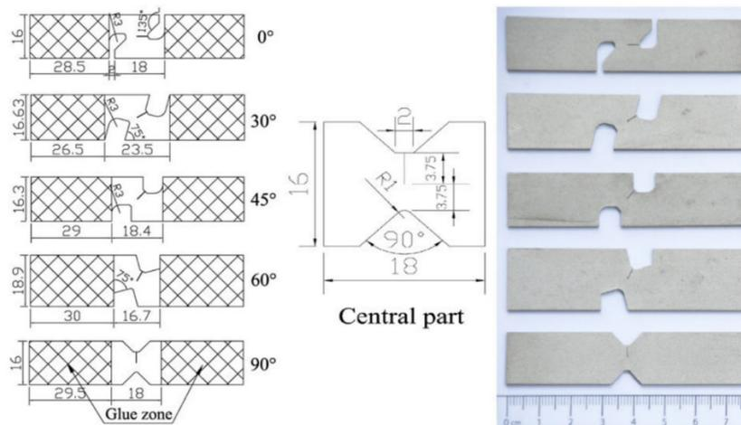
**Figure 3:** The novel specimens applied for the dynamic mixed-mode loading (Wen et al. 2016).
