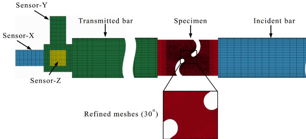
Figure 6: The finite element model scheme.
