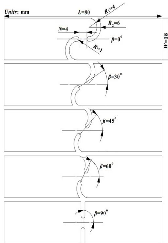
**Figure 4:** Geometry of the specimens.
