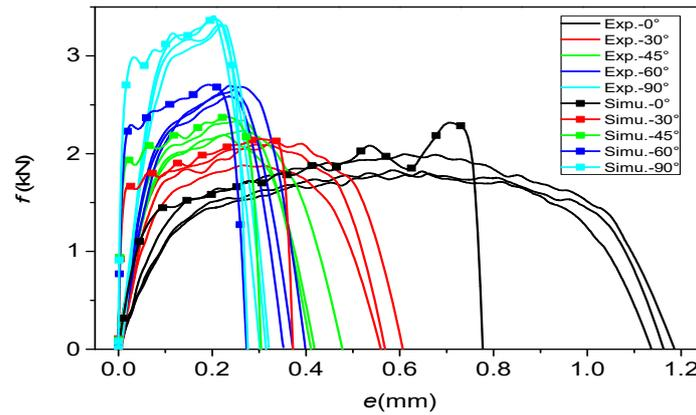
Figure 7: Comparisons of Force elongation curves of specimens with different loading angles between experiments and simulations.
