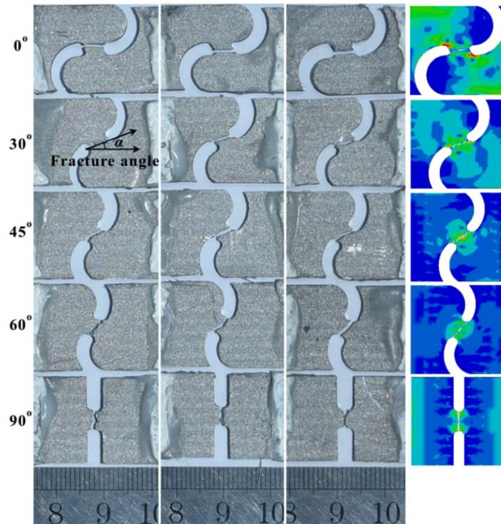
**Figure 8:** Fractured specimens of experiments and simulations.
