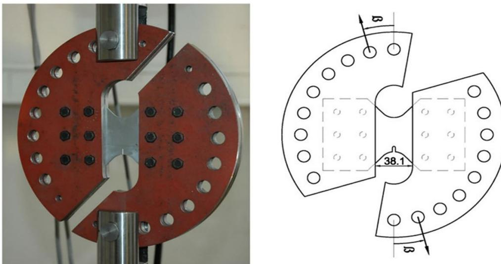
**Figure 2:** The modified Arcan specimen (Fagerholt et al. 2010).
