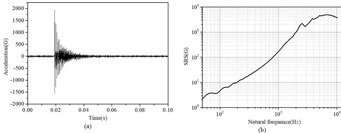
**Figure 10:** Typical shock pulse and the corresponding maximum SRS (30°-I#). (a) Acceleration data in time domain. (b) The corresponding maximum SRS.
