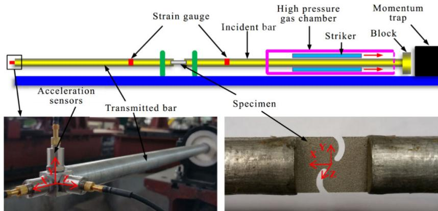
Figure 5: The sketch of the SHTB test platform.
