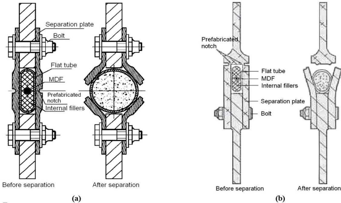
**Figure 1:** The expansion tube separation device. (a) Tensile fracture mode (Song et al., 2015). (b) Shear fracture mode (Fritz 2003).
