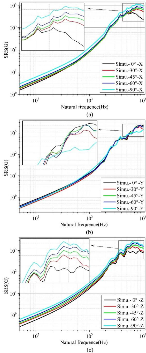
**Figure 12:** Maximum SRS in simulations. (a) X-direction. (b) Y-direction. (c) Z-direction.
