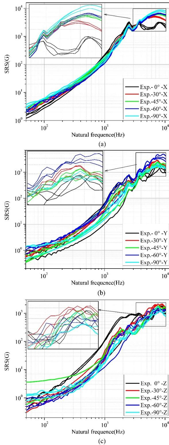
**Figure 11:** Maximum SRS in experiments. (a) X-direction. (b) Y-direction. (c) Z-direction.
