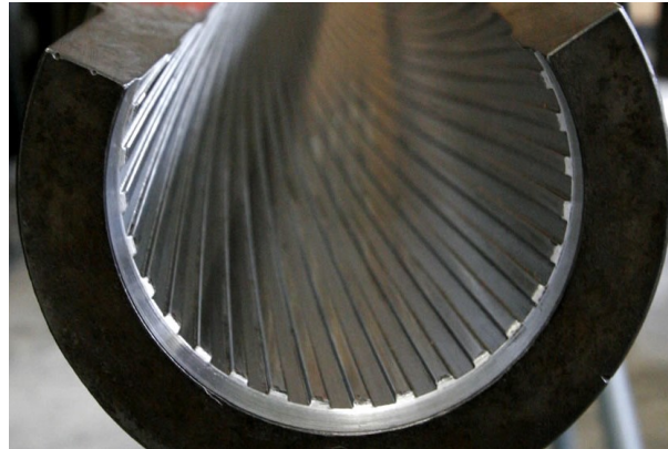
Figure 7: Groove structure of a barrel.
