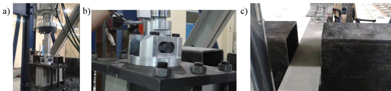
Figure 5: Some equipment used in experimental tests; a) actuator, b) connection apparatus, c) lateral supports.
