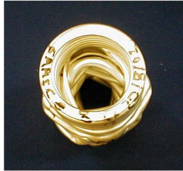
Figure 9: Internal tearing of the wrinkle at a transition between axisymmetric (concertina) deformations and the diamond mode for specimen SAASC8 [9].
