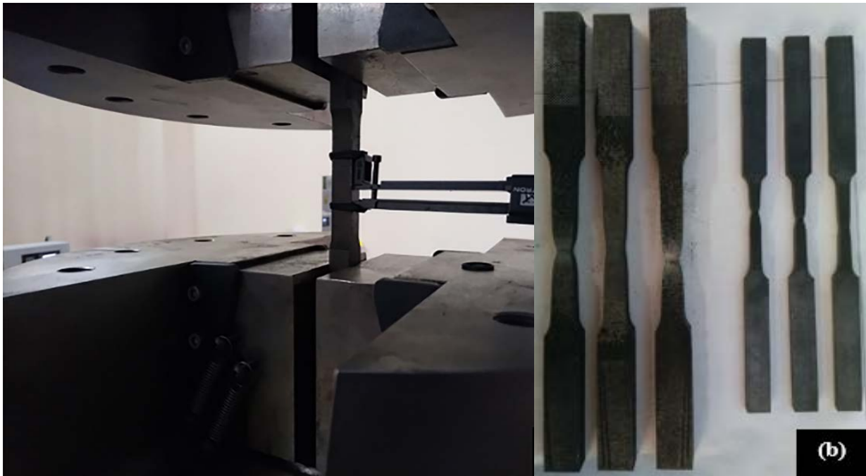
Figure 5: (a) Coupons while testing, and (b) coupons geometry following test.
