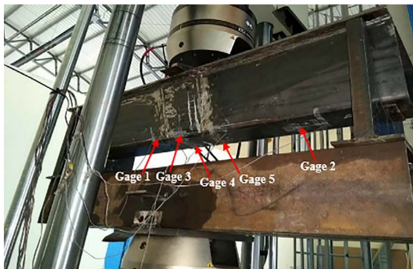
Figure 4: Gage installation in field.
