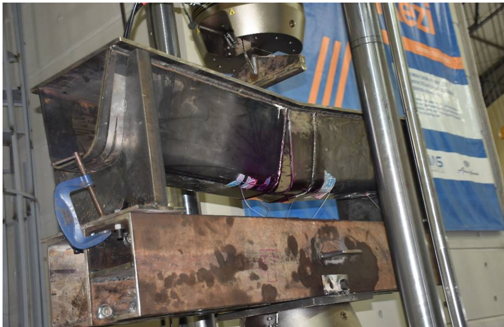
Figure 11: Failure mode at the bottom of the rib.
