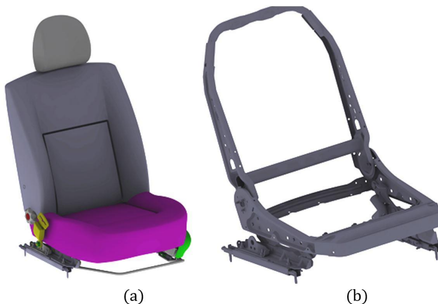
Figure 1: The seat vehicle submitted to a finite element analysis.
