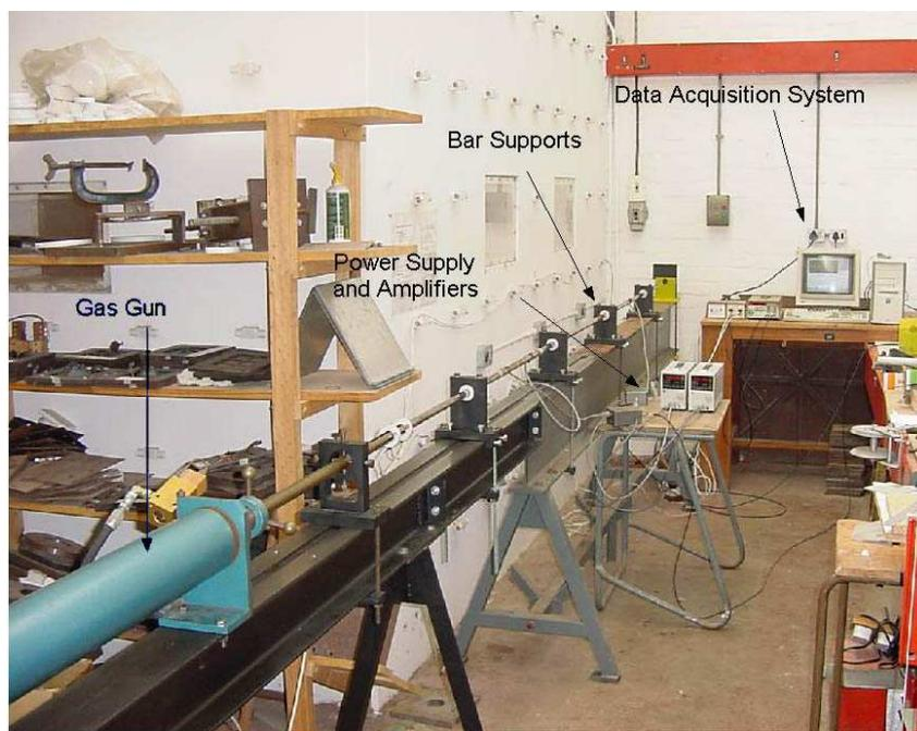
Figure 6: Photograph of the SHPB system.
