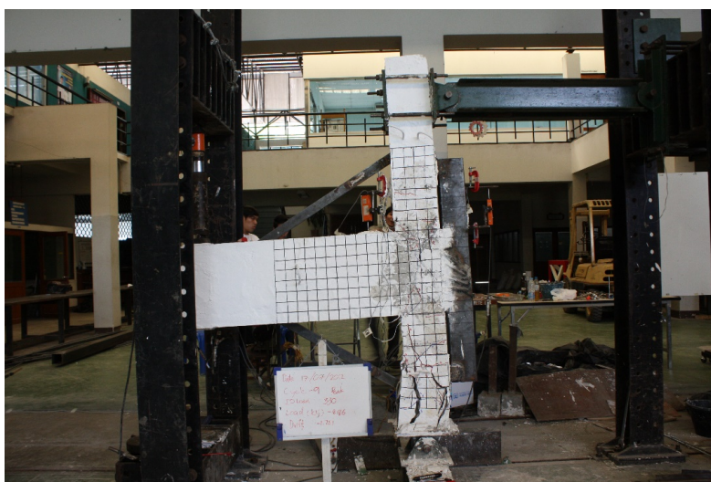
Figure 7: Failure of U5 specimen
