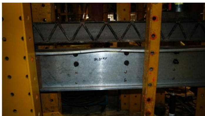
Figure 9: Typical failure mode of control specimens
