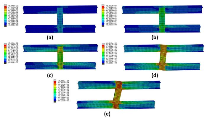
Figure 14. The MISES stress nephogram of specimen A (a)The load of 100KN; (b)The load of 200KN; (c)The load of 300KN; (d)The load of 400KN; (a)The load of 420KN;
