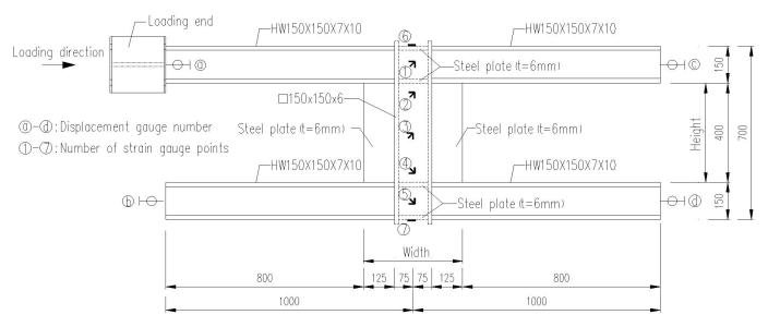
Fig.5 Dimensions of Group B and layout of measuring points
