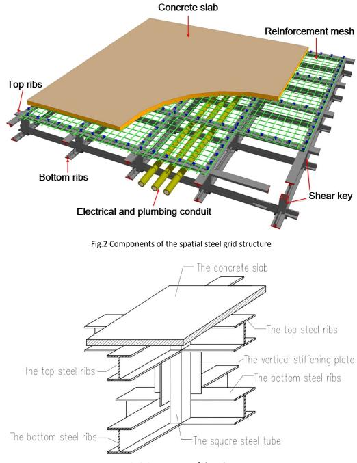
Fig.3 Components of shear key
