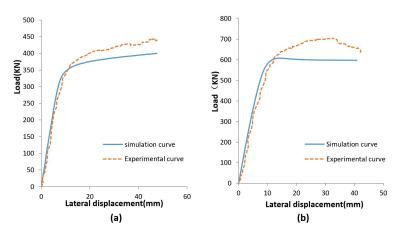
Figure 13. The comparisons of Load-Displacement Curves (a) The comparison of Load-Displacement Curve for A; (b) The comparison of Load-Displacement Curve for B.
