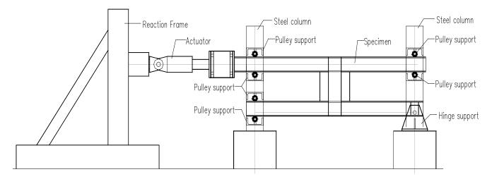
Fig.6 Schematic diagram of loading device
