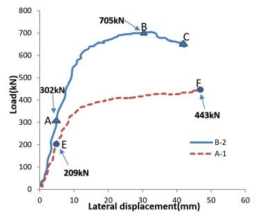
Fig.11 The loading-displacement curves of A-1 and B-2
