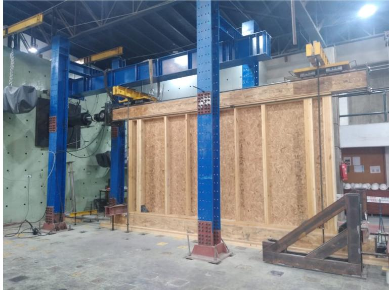
**Figure 18.** Test setup of the shear wall specimen before installing the double ELAS mechanism, dampers, and instrumentation (the blue frame shown in the picture is not part of the test setup).
