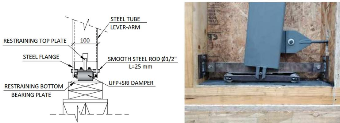
**Figure 17.** Details of the connection between the UFP+IRS damper and the lever arm of the ELAS amplification mechanism.
