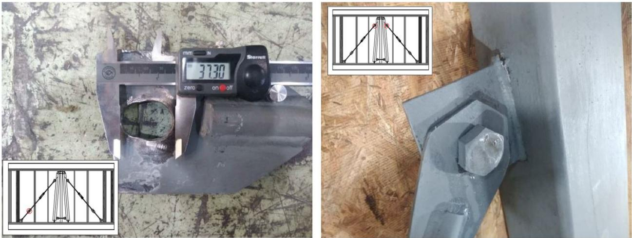
Figure 27. Plastic deformations at the connections of the amplification system due to design flaws.
