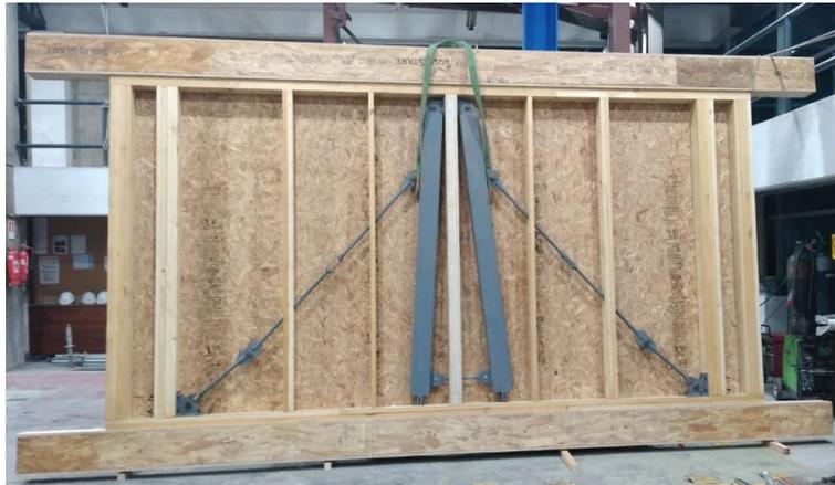
**Figure 14.** Conventional wood-frame shear wall with double ELAS mechanism prior to the experimental test and the incorporation of the dampers.
