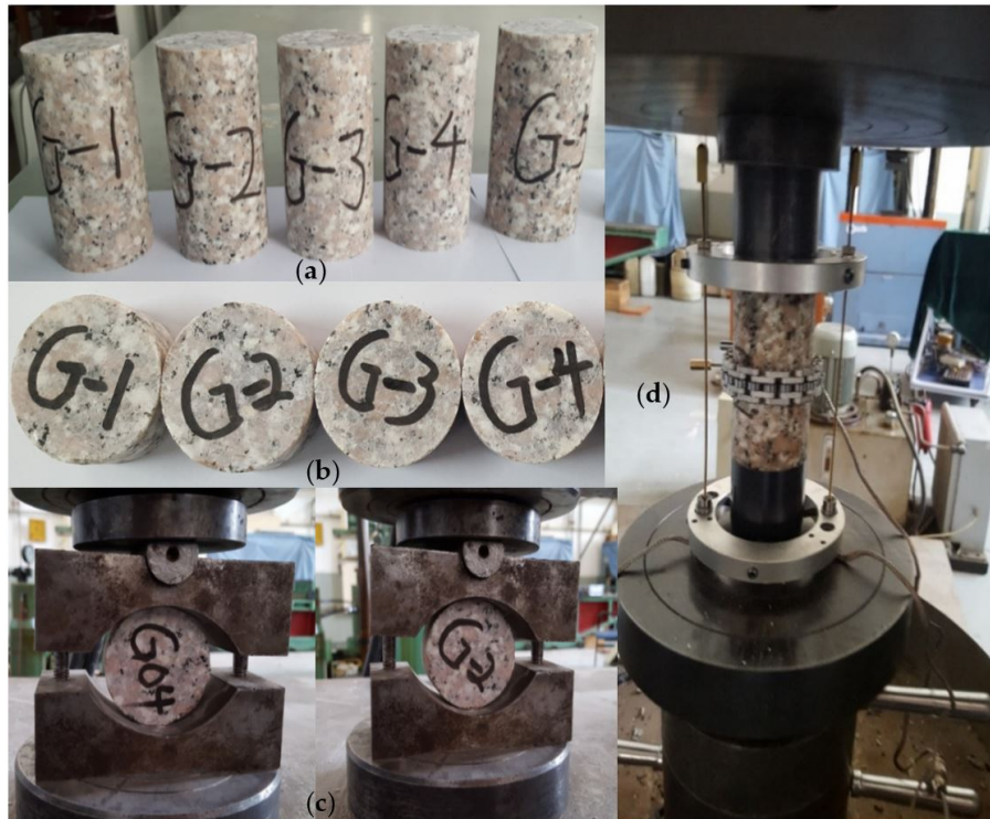
Figure 4. Rock sample for UCS test and BTS test: (a) Rock specimen for UCS test; (b) Rock specimen under UCS test; (c) Rock specimen for BTS test; (d) Rock specimen under BTS test.
