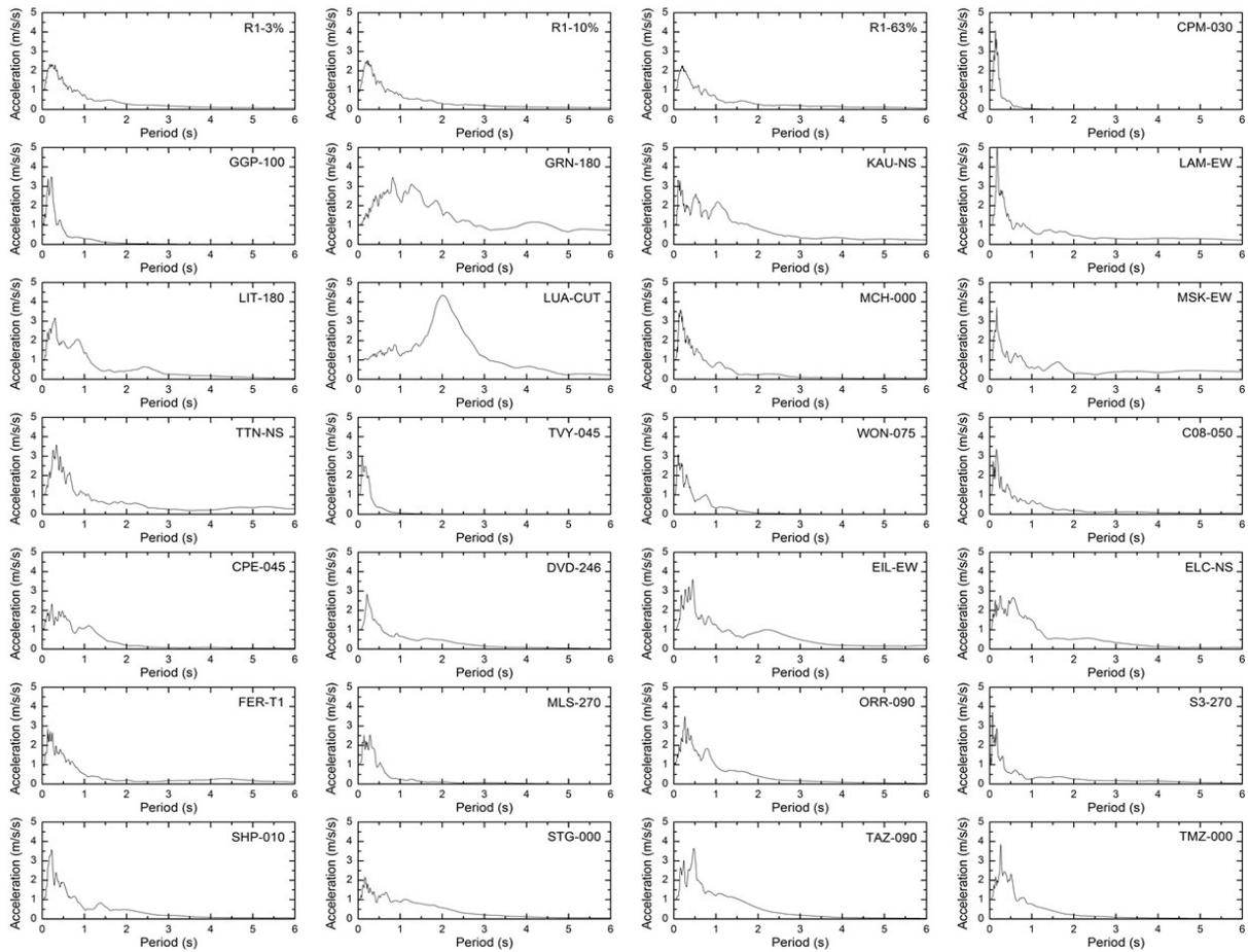
Fig.3 Acceleration response spectra (damping ratio of 0.05).
