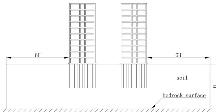
Fig.6 Arrangement of the structures and soil (CON.2).
