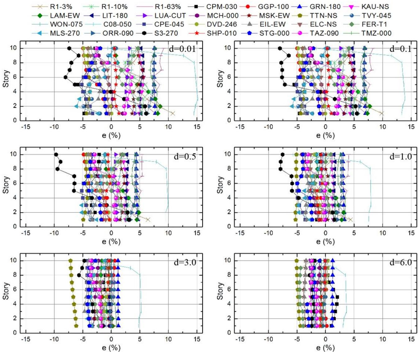
Fig.3 Influence coefficients of the story shear force at each story with different separation distances under seismic waves.
