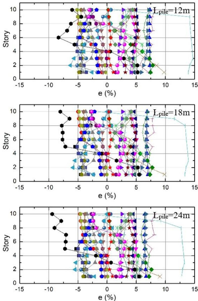
Fig.12 Influence coefficients of the story shear force at each story with different pile lengths under seismic waves.
