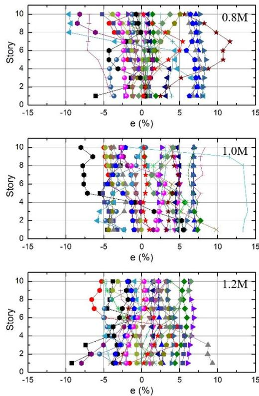
Fig.20 Influence coefficients of the story shear force at each story with different masses of the superstructure under seismic waves.
