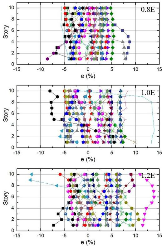
Fig.18 Influence coefficients of the story shear force at each story with different material stiffnesses of the superstructure under seismic waves.
