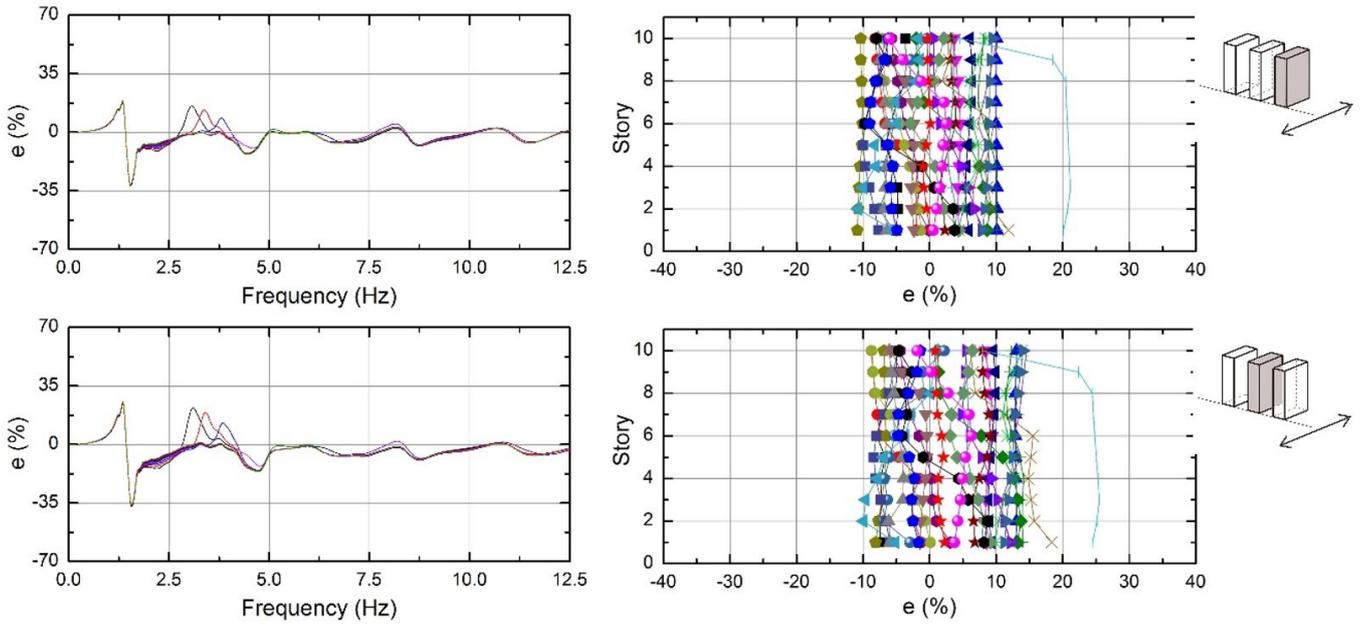
Fig.27 Influence coefficients of the story shear force at each story under harmonic waves and seismic waves. ( $N = 3$ )
