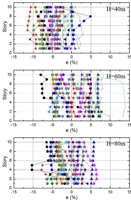
Fig.8 Influence coefficients of the story shear force at each story with different soil thicknesses under seismic waves.
