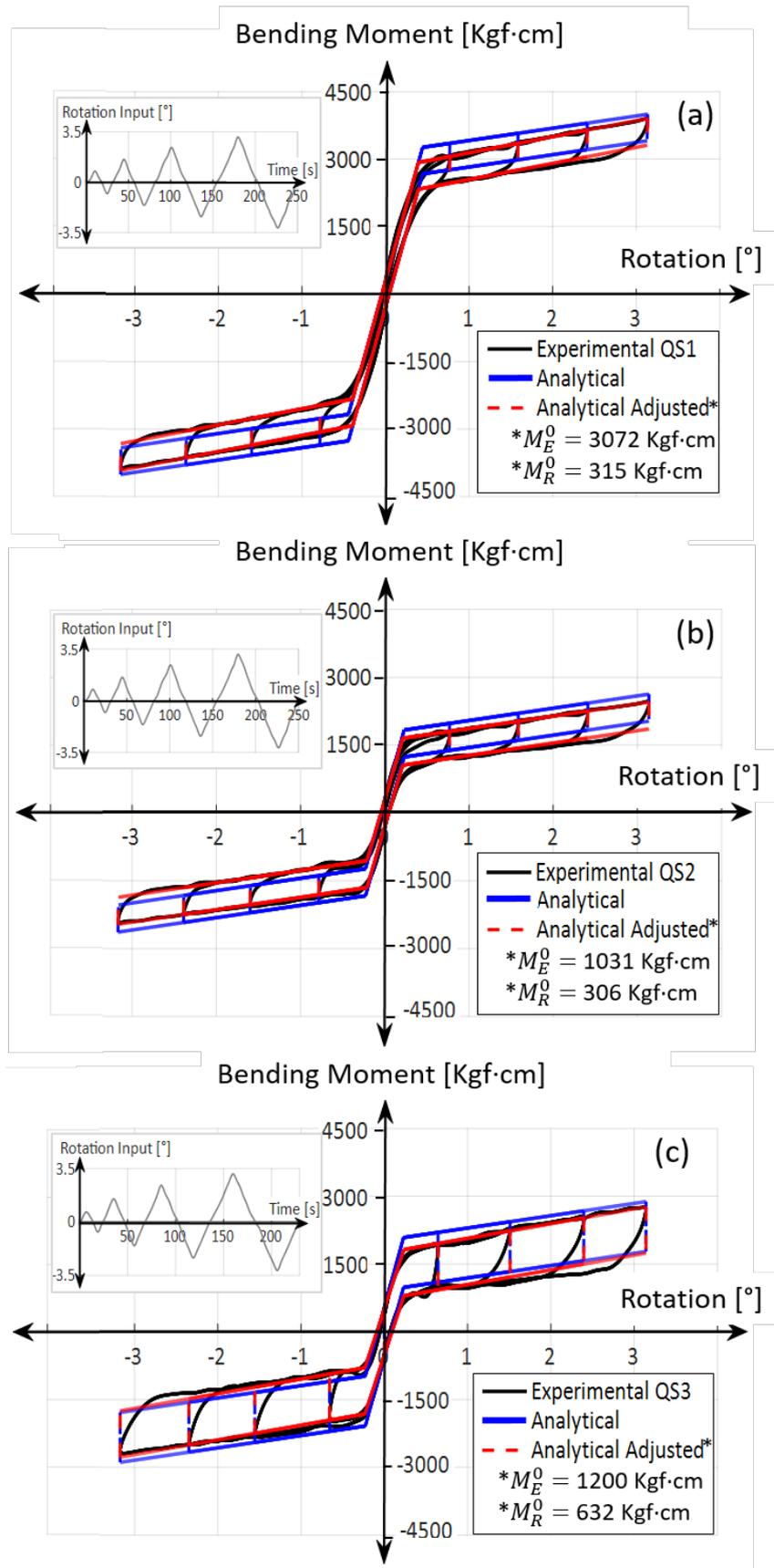
**Figure 7.** Bending moment hysteretic curves at the connection. The errors in moment at the largest rotation cycles were: (a) QS1,  $\epsilon_M^{L.C.} = 5.4\%$ ; (b) QS2,  $\epsilon_M^{L.C.} = 5.1\%$ ; (c) QS3,  $\epsilon_M^{L.C.} = 6.0\%$ . Parameters of tests QS1, QS2, QS3, in Table 1
