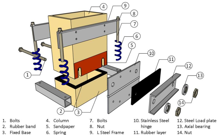
Note: Parts 10, 11, 12, 13 and 14 are also symmetrically located on the back of the structure.
