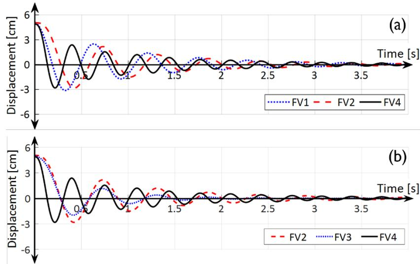
**Figure 8.** Displacement at the top column of the free vibration damping tests. (a) Different spring tension and equal bolt torque; (b) Equal spring tension and different bolt torque.
