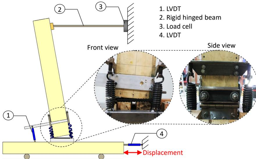
Figure 6. Arrangement of the column and the connection for the quasistatic loading tests.
