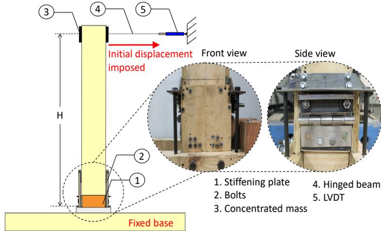
Figure 5. Arrangement of the column and the connection for the free vibration damping tests.
