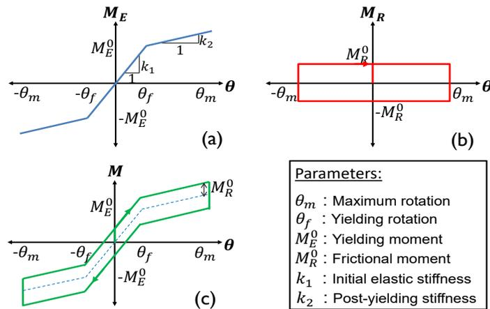
Figure 3. (a) Elastic bilinear behavior; (b) frictional behavior; (c) hysteretic curve of the device.
