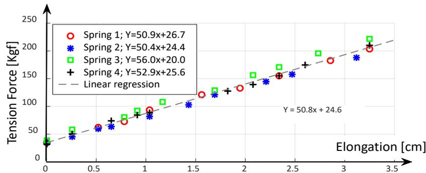
Figure 4. Load-Elongation spring curve tests.
