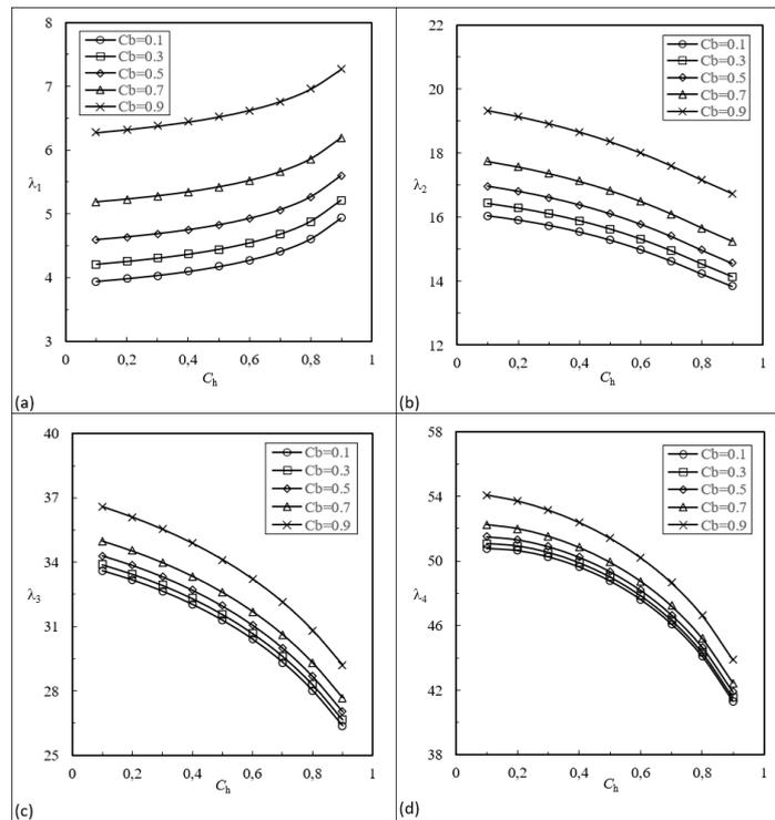
Figure 3: Effect of  $C_h$  on dimensionless natural frequencies for clamped-free Z/A AFGM beams of  $r = 0.01$  and  $\alpha = -10$  with various values of  $C_b$ . (a) First mode (b) Second mode (c) Third mode (d) Fourth mode
