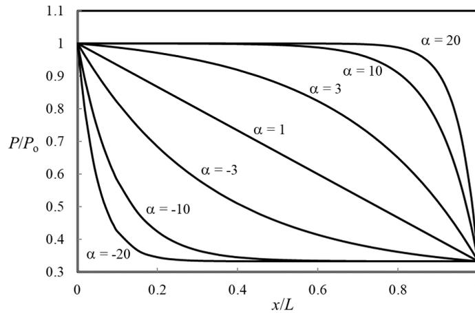
**Figure 2:** Variation of effective property  $P(x)/P_0$  versus beam length for exponentially AFGM beam with various values of material graded index  $\alpha$ .
