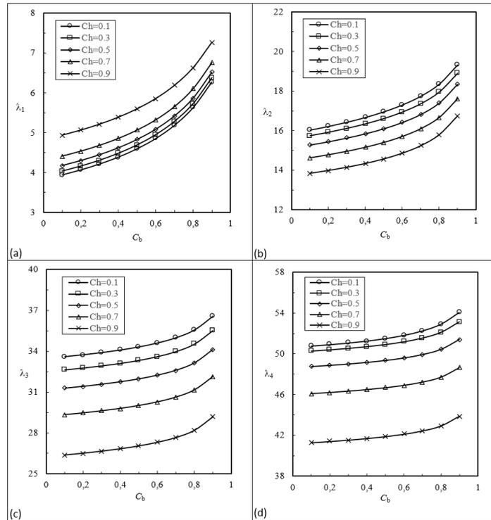
Figure 4: Effect of  $C_b$  on dimensionless natural frequencies for clamped-free Z/A AFGM beams of  $r = 0.01$  and  $\alpha = -10$  with various values of  $C_h$ . (a) First mode (b) Second mode (c) Third mode (d) Fourth mode.
