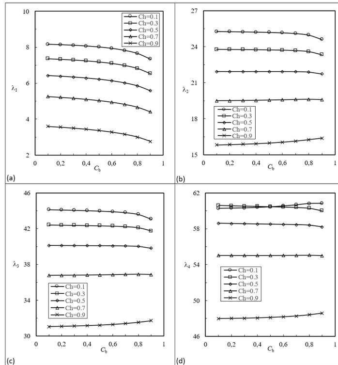
**Figure 6:** Effect of  $C_b$  on dimensionless natural frequencies for pinned-pinned Z/A AFGM beams of  $r = 0.01$  and  $\alpha = -10$  with various values of  $C_h$ . (a) First mode (b) Second mode (c) Third mode (d) Fourth mode.
