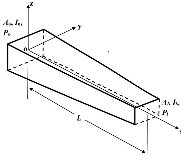
Figure 1: Axially FGM beam configuration and coordinate systems.
