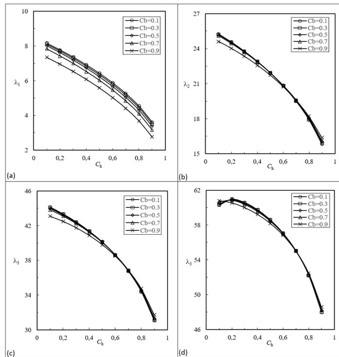
Figure 5: Effect of  $C_h$  on dimensionless natural frequencies for pinned-pinned Z/A AFGM beams of  $r = 0.01$  and  $\alpha = -10$  with various values of  $C_b$ . (a) First mode (b) Second mode (c) Third mode (d) Fourth mode.
