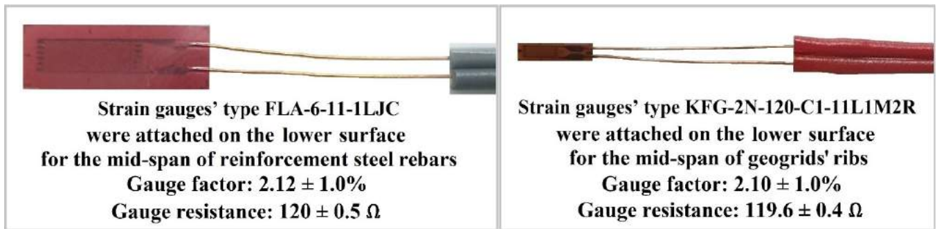
Figure 4. Types of utilized strain gauges.
