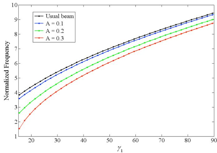
Figure 7 Comparison of usual beam and quintic nonlinear beam as a function of  $\gamma_1$
