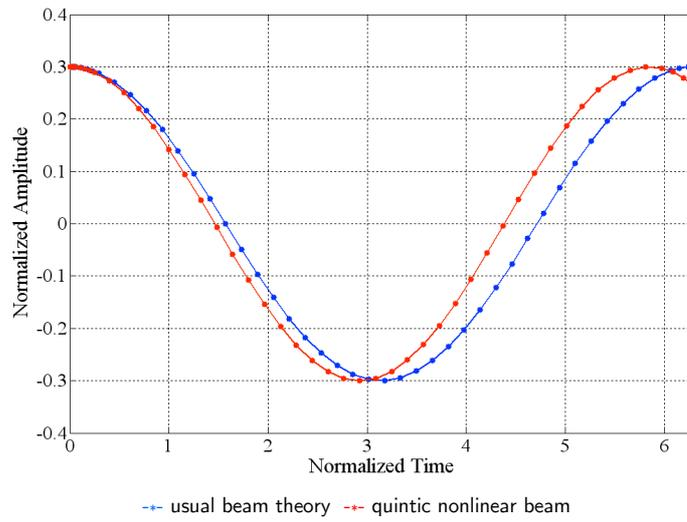
Figure 4 The impact of nonlinear terms on the beam dynamical behavior for  $A = 0.3$  and  $\gamma_1 = 80$
