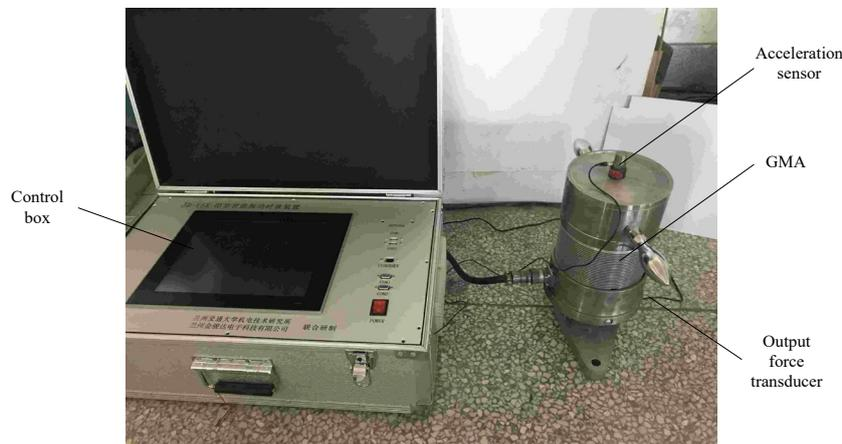
Figure 2. Physical picture of GMA test system.
