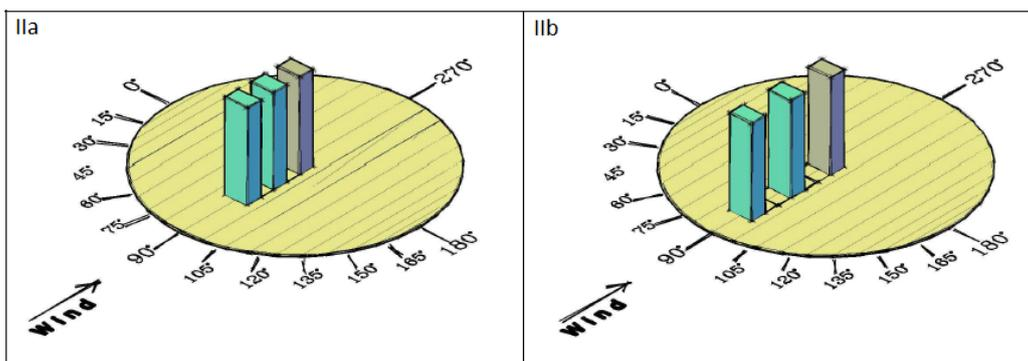
Figure 2 Perspectives of tests and wind incidence angles in Configuration II
