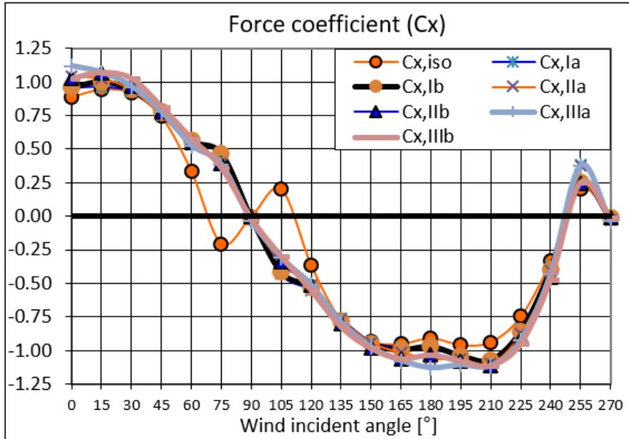
Figure 10 Force Coefficient (Cx) in all configurations
