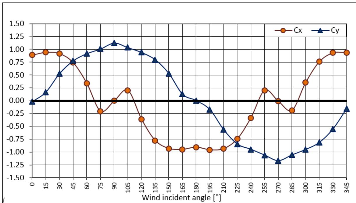
Figure 9 Force coefficients (Cx and Cy) in the Isolated Configuration
