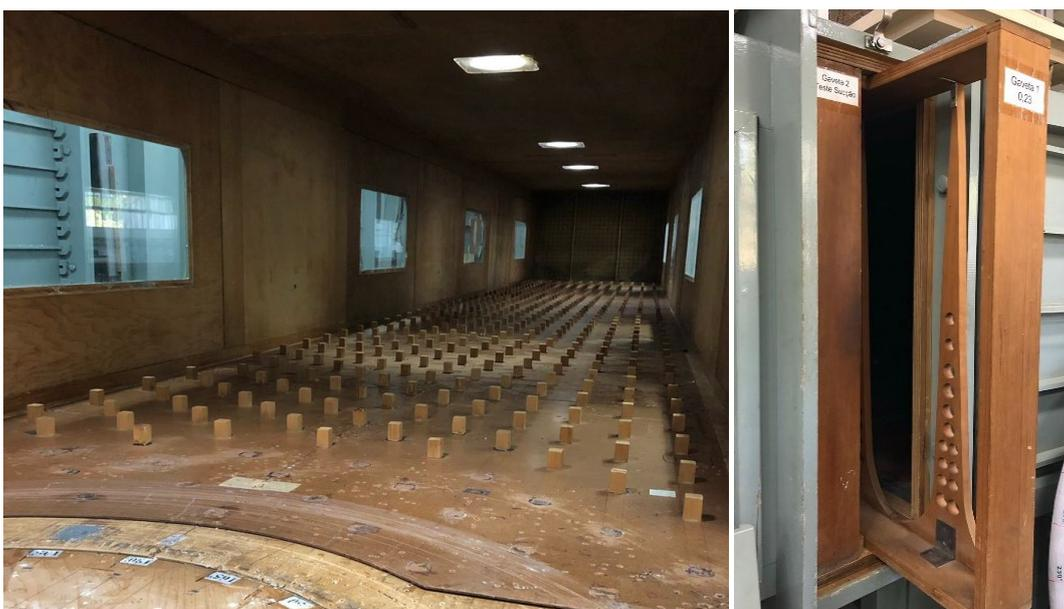
**Figure 8** Devices inside the tunnel to simulate the profile with exponent  $p = 0.23$
