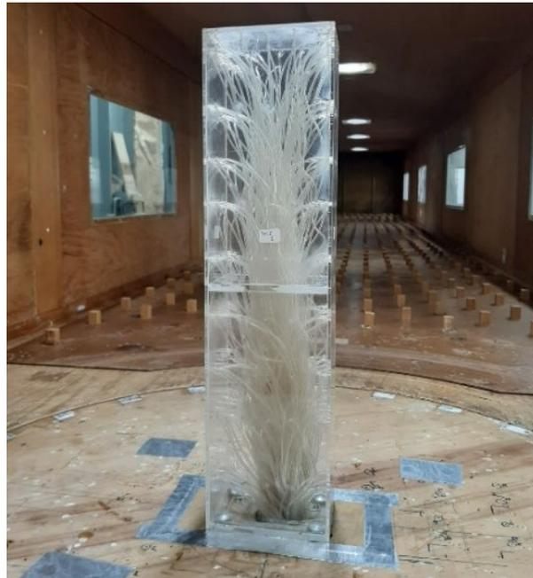
**Figure 5** Reduced model of CAARC inside the Wind Tunnel Prof. Joaquim Blessmann
