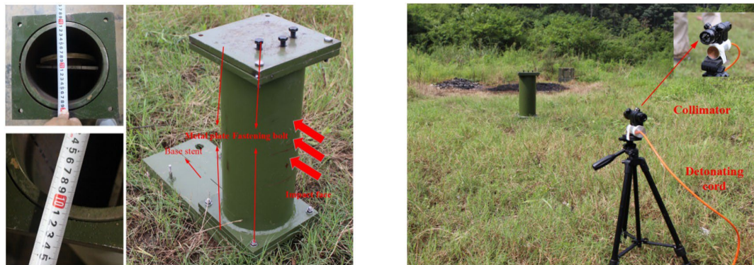
Figure 22: Test settings of the simulated target and EFP-warhead impact detonating simulated target
