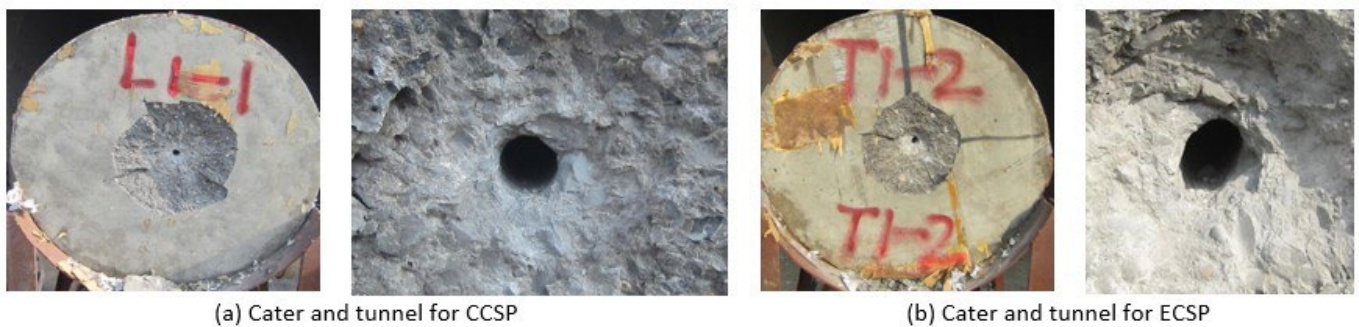
Figure 5. Damage of concrete targets.
