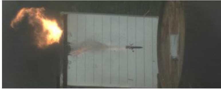
Figure 3. Attitude of E1 projectile in Test NO.7.
