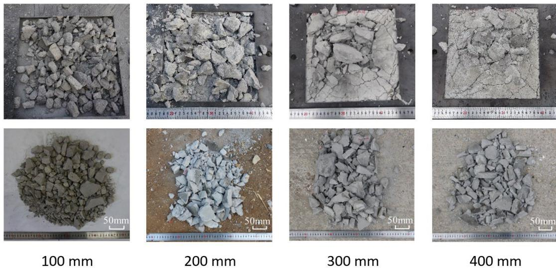
Figure 4 Fracture and fragmentation of foam concrete plates with different stand-offs (the plate thickness is 20mm)
