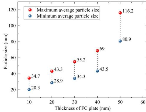
**Figure 8** Fragments size of foam concrete plates with different thicknesses
