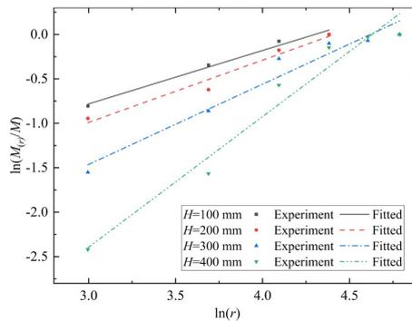
Figure 13 Fractal dimension of foam concrete fragments with different stand-offs
