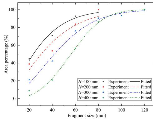
**Figure 9** Cumulative probability of fragments area of foam concrete with different stand-offs
