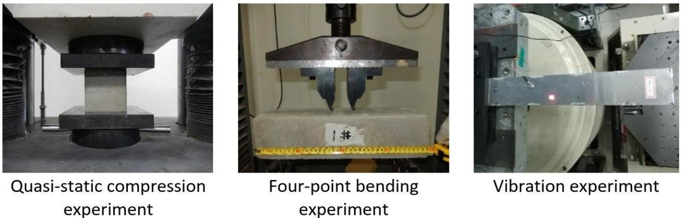
Figure 1 Mechanical properties test of foam concrete
