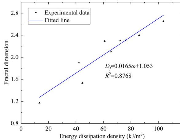
**Figure 17** Relationship between fragmentation fractal dimension and energy dissipation density
