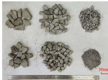
**Figure 11** Size distribution of foam concrete fragments(400 mm stand-off / 20 mm plate thickness)
