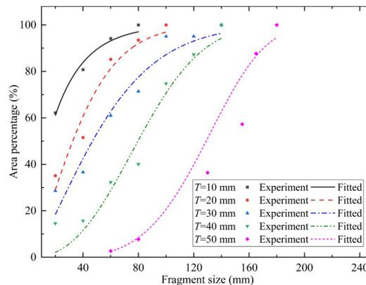
**Figure 10** Cumulative probability of fragment area of foam concrete with different plate thicknesses
