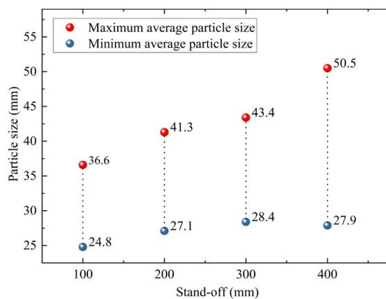
Figure 7 Fragments size of foam concrete plates with different stand-offs
