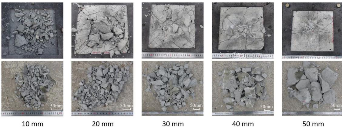
Figure 5 Fracture and fragmentation of foam concrete plates with different plate thicknesses (the stand-off is 300 mm)
