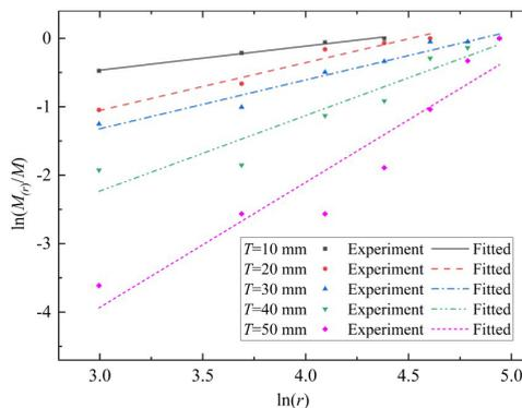
Figure 14 Fractal dimension of foam concrete fragments with different plate thicknesses
