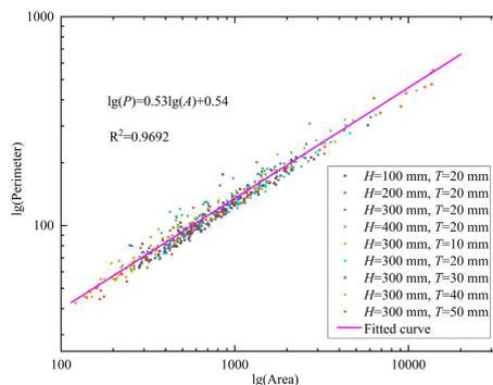
**Figure 12** Perimeter and area distribution of foam concrete fragments
