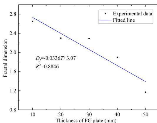
**Figure 16** Relationship between fragmentation fractal dimension and plate thickness
