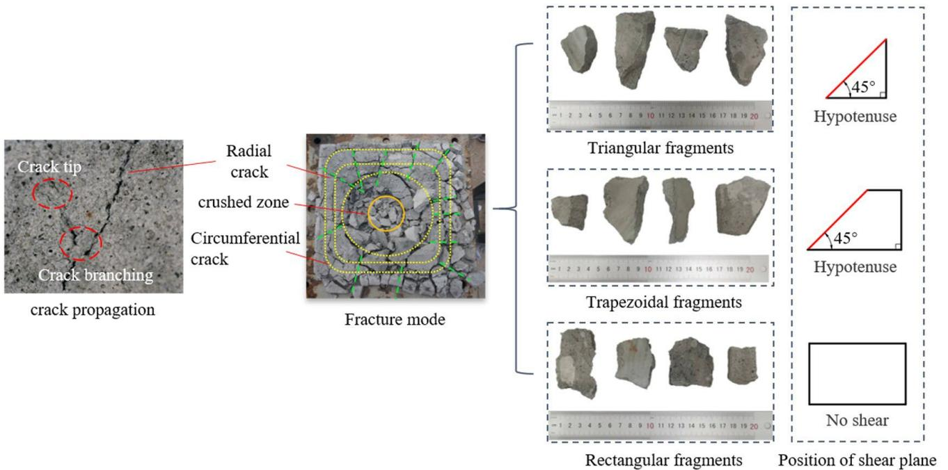
Figure 3 Analysis of fragmentation process and fracture morphology of foam concrete
