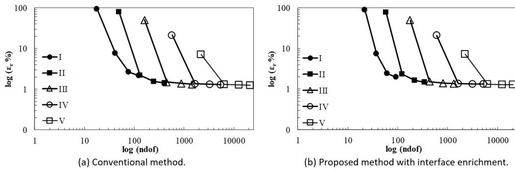
**Figure 8** Relative error,  $\varepsilon_r$ , with respect to the ndof for each mesh by adding enrichment functions at different degrees on each mesh for determining the strain energy.
