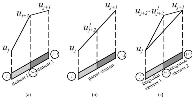
**Figure 2** Approaches in a domain with 2 materials. (a) Conventional FEM interpolation; (b) Interpolation with a non-conforming element; (c) Interpolation using the proposed method with interface enrichment.
