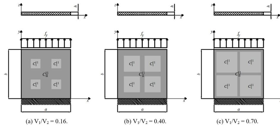
**Figure 9.** Geometry and loading of the composite model for different volume relations
