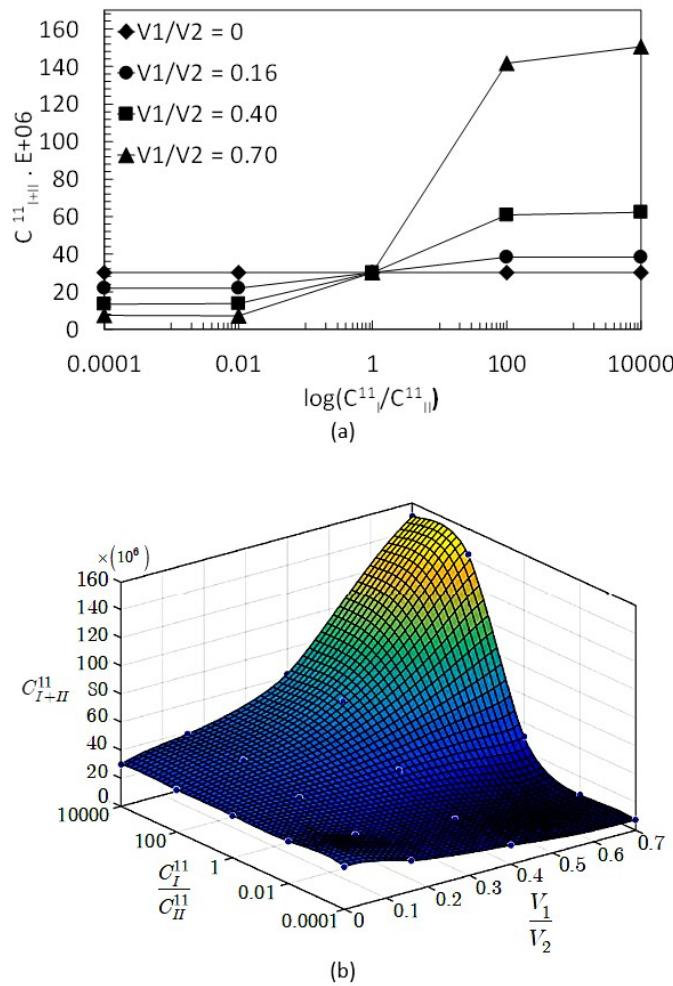
**Figure 13**  $C_{I+II}^{11}$  Value in mesh for different relations of  $C_I^{11}/C_{II}^{11}$  and proportions between volumes.
