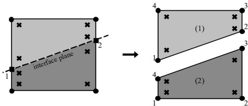
**Figure 4** Evaluation of enrichment functions in the proposed method with interface enrichment for quadrilateral elements.
