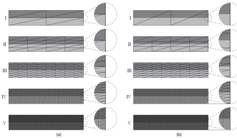
**Figure 6.** Different mesh configurations for the two-materials-composited beam: (a) the conventional method; (b) the proposed method with interface enrichment.
