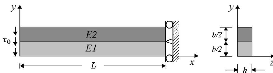
**Figure 5.** Geometry and loading of the two-material-composed beam subjected to simple bending.
