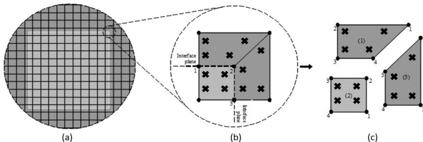
**Figure 11** Enrichment functions in 2D of the proposed method with the creation of integration elements for four-node quadrilateral elements, cut by an interface made by two line segments intercepted.
