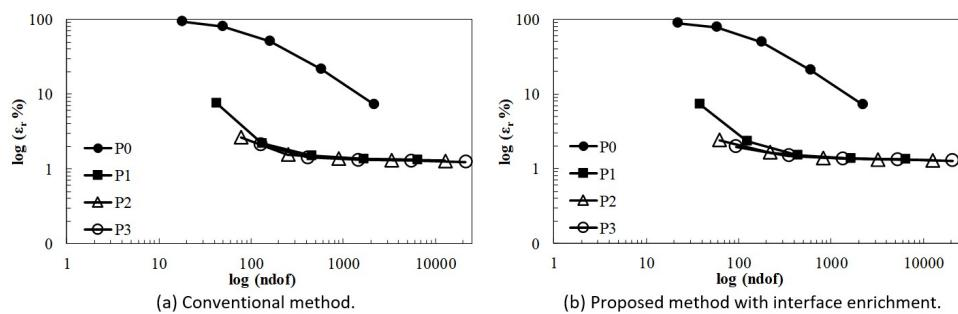
**Figure 7** Relative error  $\varepsilon_r$ , for the strain energy in relation to the ndof for different degrees of enrichment functions to the relationship  $E_1/E_2 = 10$ .
