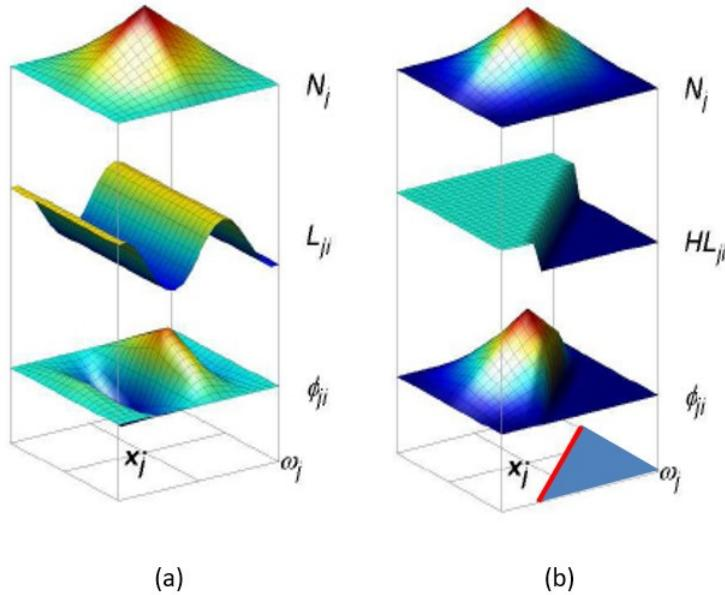
**Figure 1** Construction of the proposed enrichment method's shape functions (a) continuous; (b) high-order discontinuous (Evangelista Jr. et al., 2020).
