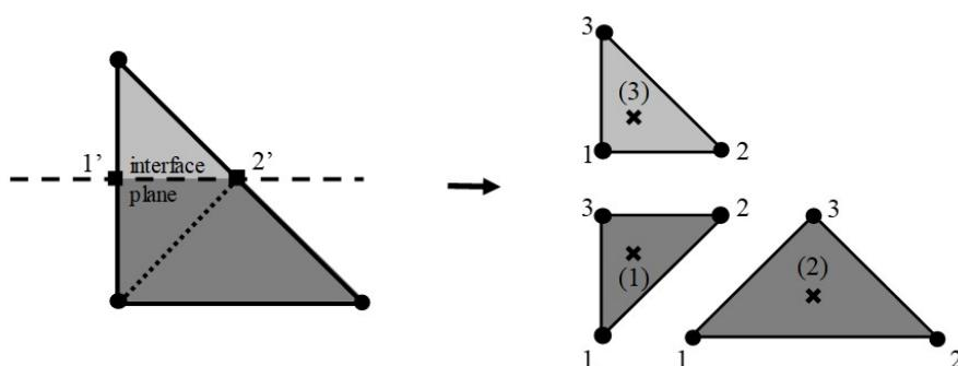
**Figure 3** Evaluation of enrichment functions in the proposed method with interface enrichment for triangular elements.
